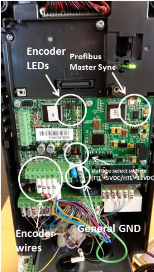
Figure 2 – C2000 with encoder card and Profibus card with no active Master in the system
