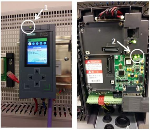
Figure 33 – 1 – Master, 2 - Slave cyclic communication established
