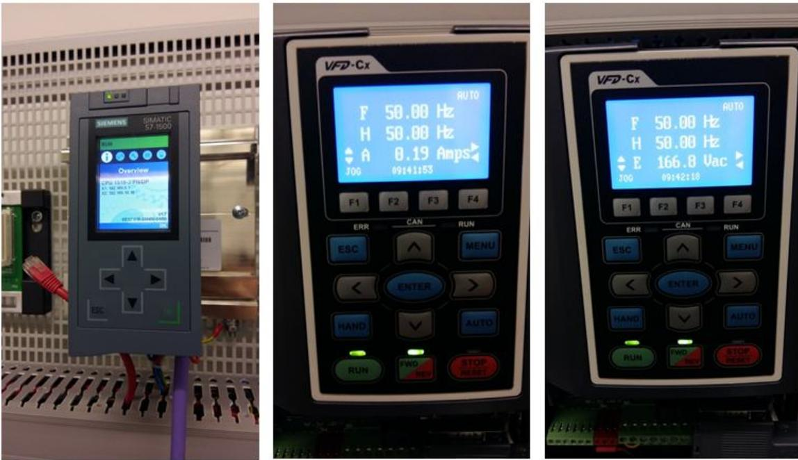
Figure 54 - Profibus Master sending and receiving, drive runs and current, frequency and voltage are displayed
