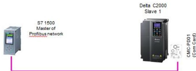
Figure 3 - Example of our first Profibus network example with S7 1500 Master and Slave.
