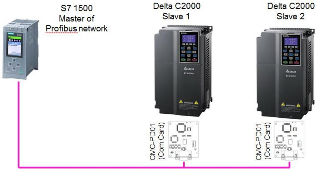
Figure 1 - Topology of a Profibus Network with the Master and 2 Slave peripherals.
