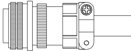
ASDBCAPW0100 (for 200V drives, with brake cable)
