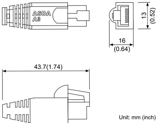
• **A3 CN6 DMCNET Termination Resistor**
