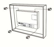
Step 4: For heat dissipation, please keep a minimum clearance of 60 mm on the rear of the HMI.
