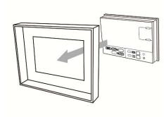
Step 3: Tighten the screws with the torque less than 0.5 N-M / 0.7 N-M to avoid damage to the plastic case.
