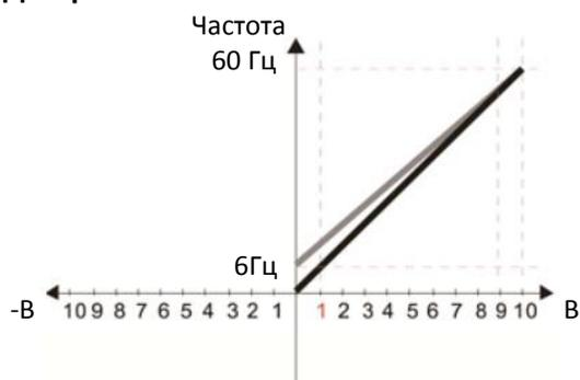
$$\frac{60-6\text{Гц}}{10\text{В}} = \frac{6-0\text{Гц}}{(0-x\text{В})}; x\text{В} = \frac{100}{-9} = -1.11\text{В};$$
