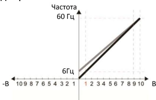
$$\frac{60-6\text{Гц}}{10\text{В}} = \frac{6-0\text{Гц}}{(0-x\text{В})}; x\text{В} = \frac{100}{-9} = -1.11\text{В};$$
