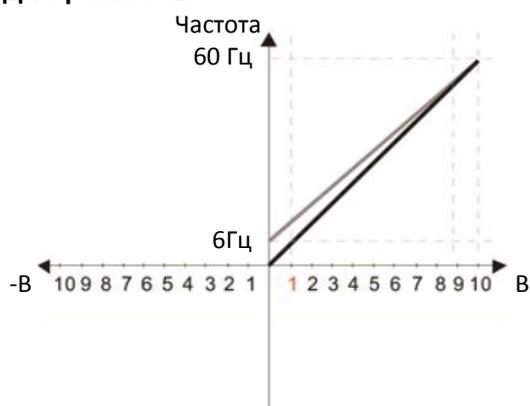
$$\frac{60-6\text{Гц}}{10\text{В}} = \frac{6-0\text{Гц}}{(0-x\text{В})}; x\text{В} = \frac{100}{-9} = -1.11\text{В};$$
