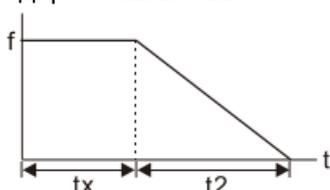
$$S = n \times \left( \frac{t_x + (t_x + t_2)}{2} \right)$$
