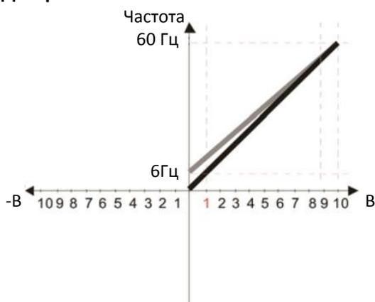
$$\frac{60-6\text{Гц}}{10\text{В}} = \frac{6-0\text{Гц}}{(0-x\text{В})}; x\text{В} = \frac{100}{-9} = -1.11\text{В};$$
