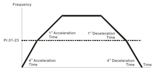
1<sup>st</sup>/4<sup>th</sup>Acceleration/Deceleration Frequency Switching
