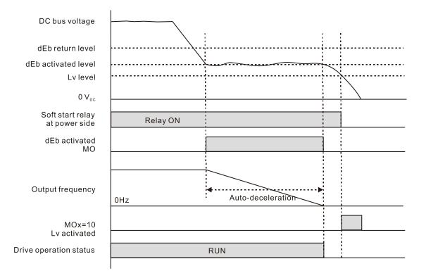
Situation 4: Pr.07-13 = 2 and power does not recover, same situation as Situation 3. The drive decelerates to 0 Hz. The DC bus voltage continues to decrease until the voltage is lower than the Lv level, and then the drive disconnects the soft start relay. The keypad displays "dEb" warning until the drive completely runs out of power.
