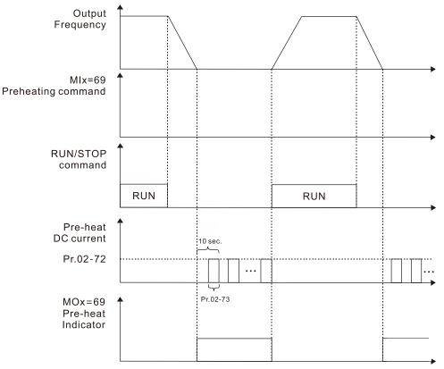
The figure below shows the timing relationship when MI=69 enable preheating function is disabled and when preheating DC current is enabled and cycle time is 50%. When the motor drive is stopped, the preheating function starts to output DC current continuously.
