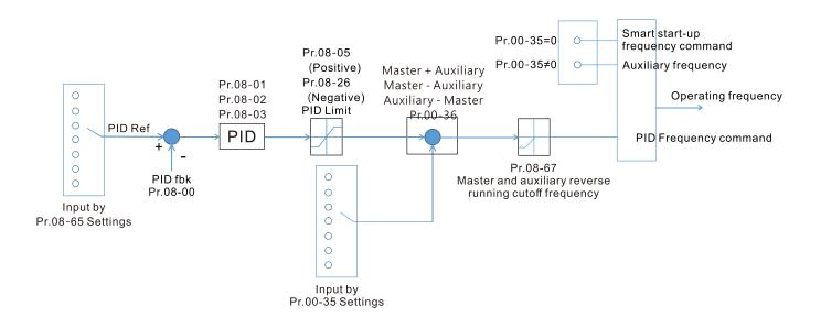
$\square$  When Pr.08-65  $\neq$  0, the PID controller architecture shows as the diagram below:
