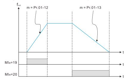
When Pr.02-09 is set to 1: The increasing or decreasing Frequency command (F) operates according to the setting of Pr.02-10 (0.01–1.000 Hz/ms).
