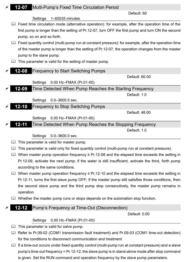
Definition to re-detect if a slave pump is time-out.
