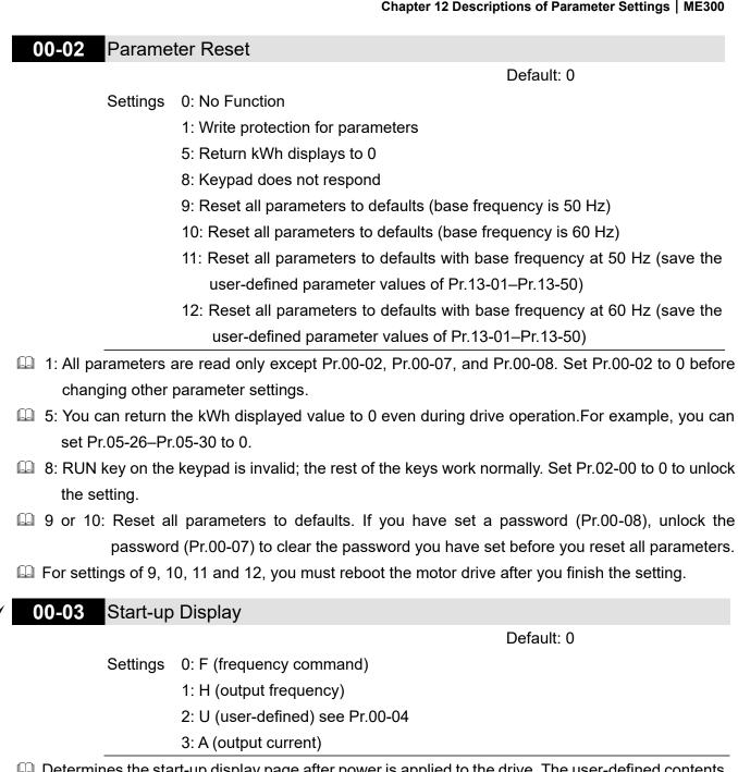
Determines the start-up display page after power is applied to the drive. The user-defined contents display according to the Pr.00-04 settings.
