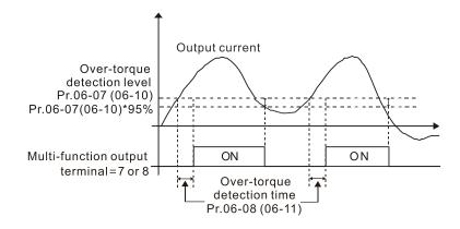
When you set Pr.06-06 or Pr.06-09 to 2 or 4, an ot1 / ot2 fault displays and the drive stops running after over-torque detection. The drive does not run until you manually reset it.
