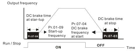
DC Brake Output Timing Diagram
