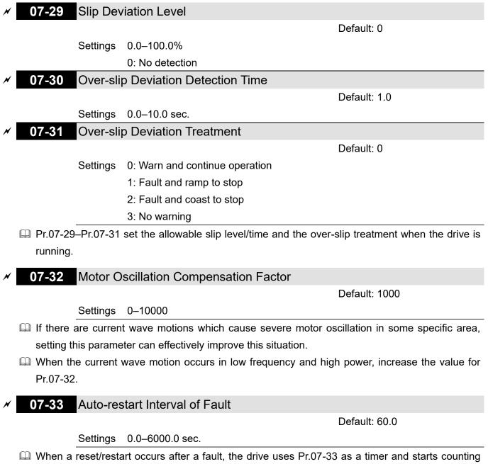
When a reset/restart occurs after a fault, the drive uses Pr.07-33 as a timer and starts counting the number of faults within this time period. Within this period, if the number of faults does not exceed the setting for Pr.07-11, the counting clears and starts from 0 when the next fault occurs.
