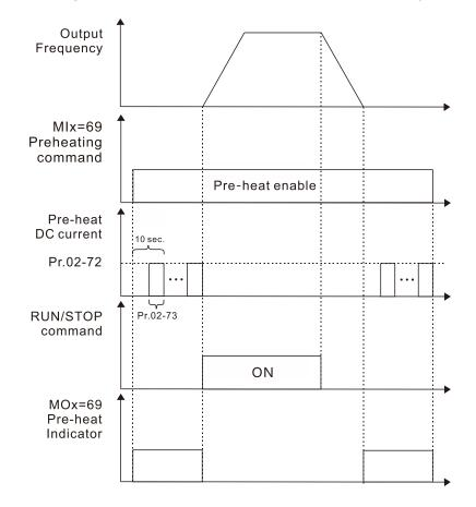
The figure below shows the timing relationship between preheating function and enabling DC brake.
