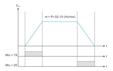
When Pr.02-09 is set to 2: The increasing or decreasing Frequency command (F) operates according to the pulse of Pr.02-10.
