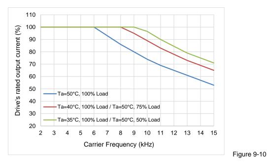
The rated output current (unit: %) of DPWM in different carrier frequencies with heavy duty.
