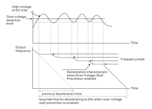
When you set Pr.06-02 to 1 to use smart over-voltage stall prevention during deceleration, the drive maintains the DC bus voltage when decelerating and prevents the drive from OV.
