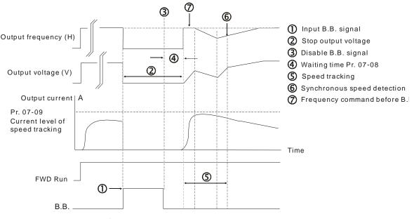
B.B. Speed tracking: from last output frequency
