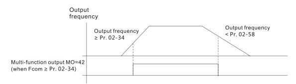
It is recommended that you use this with the Dwell acceleration/deceleration function as shown in the following diagram.
