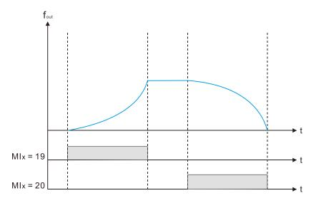
When Pr.02-09 is set to 4: The increasing or decreasing Frequency command (F) operates according to the setting of Pr.02-10 for every 100 ms.
