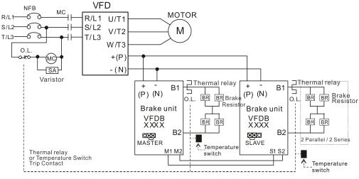
When AC Drive is equipped with a DC reactor, please read user manual for the correct wiring for the brake unit input circuit +(P).
