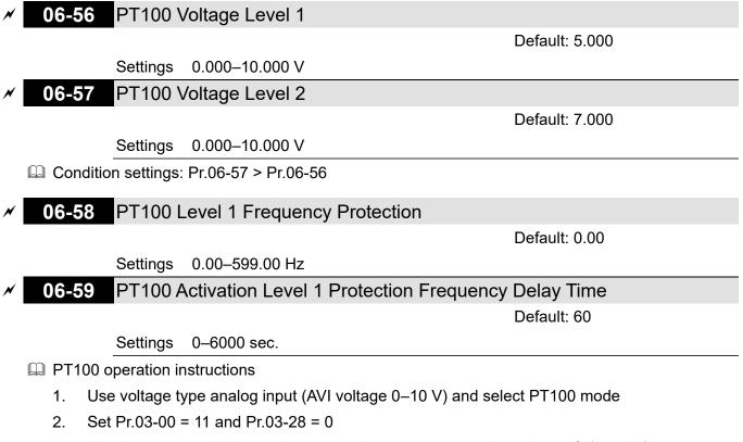
3. Need to connect divider resistance and recommended voltage is  $950\Omega \ge 0.2W$ .
