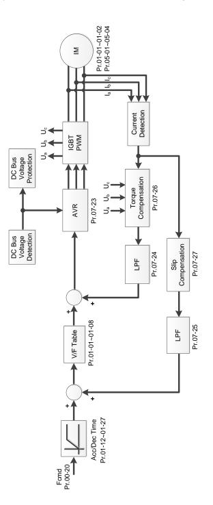
When Pr.00-10 = 0 and you set Pr.00-11 to 2, the sensorless vector control diagram is as follows: IM Space Vector Control (IMSVC)
