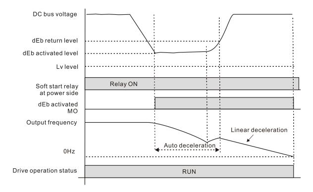
Situation 2: Momentary power loss, or too low and unstable power voltage, or power supply sliding down because of sudden heavy load
