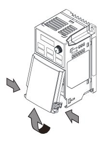
Press the clip on both sides, and then remove the cover by rotating it.
