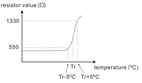
Refer to the following calculation when Pr.06-30 is set to 23% and motor temperature overheating protection level is 1330  $\Omega$ :
