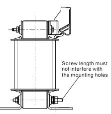
Tightening torque 0.6-0.8Nm
