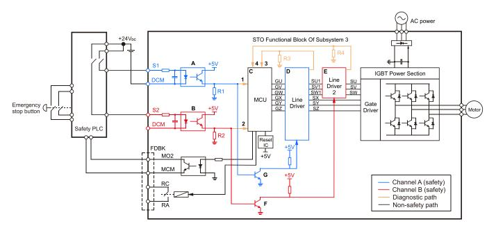
Figure 15-1 The circuit diagram for STO function
