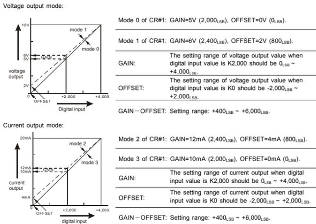
The charts above are D/A conversion characteristic curve of voltage input mode and current input mode. Users can adjust above characteristic curve by changing OFFSET values (CR#18 ~ CR#21) and GAIN values (CR#24 ~ CR#27) depend on application.
