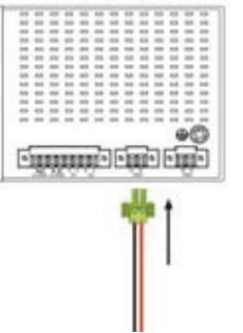
NOTE: Grounding the ground terminal on the DVS series switch can avoid the noise effect due to the electromagnetic interference (EMI).
