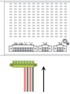
The electrical circuit of DI1 and DI2 are independent, so you don't need to care about NPN type or PNP type of DI. If the electrodes positive and electrodes negative of DI has been reversed when you plug the cable, DI still can work properly.
