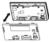
Step 3: Complete the following steps, ① and ② to replace a battery.
