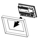
Turn the screw with less than torque 0.7N.M to avoid Keep at least 60mm distance from rear of HMI damage to plastic box.
