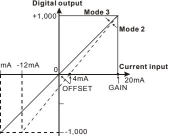
The user can adjust the OFFSET/GAIN curve of voltage/current input mode according to the actual needs by changing the OFFSET value (CR#18 ~ CR#21) and GAIN value (CR#24 ~ CR#27).
