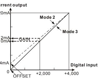
The user can adjust the OFFSET/GAIN curve of voltage/current output mode according to the actual needs by changing the OFFSET value (CR#14 ~ CR#15) and GAIN value (CR#18 ~ CR#19).
