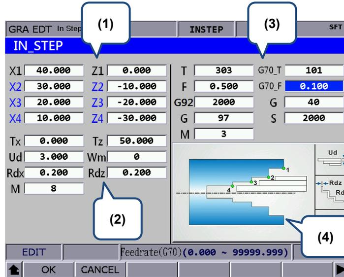
(1) Input the coordinates of each step point (Fields with blue texts can be left blank and it means the point does not exist. )
