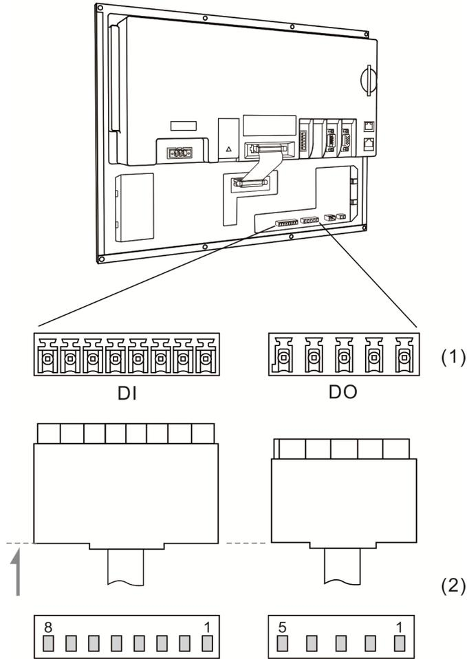
(1) Local I/O connector on NC controller (Female); (2) Local I/O connector (Male)
