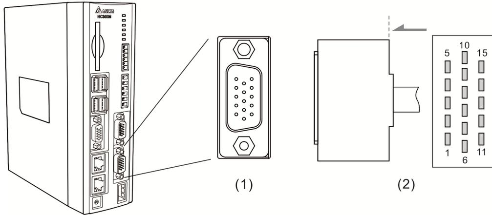
(1) Spindle connector on NC controller (Female); (2) Spindle connector (Male)
