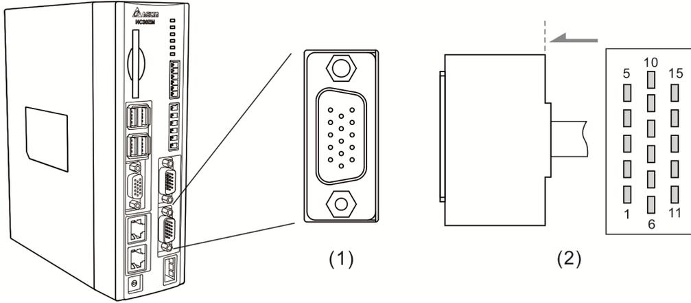
(1) RS-485 connector on NC controller (Female); (2) RS-485 connector (Male)
