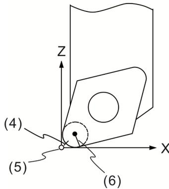
(4) Actual tool nose; (5) The assumed tool nose position when calibration;
