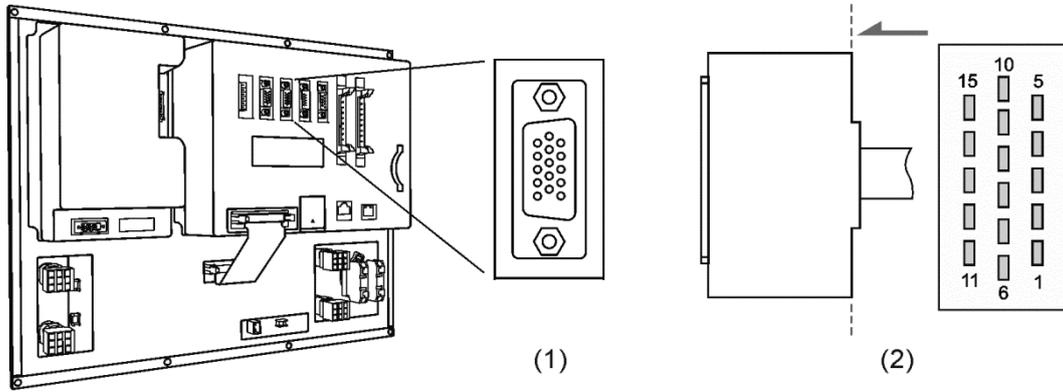
(1) Spindle connector on NC controller (Female); (2) Spindle connector (Male)
