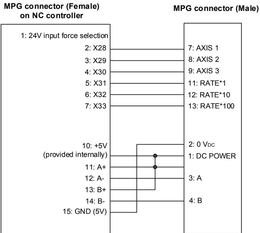
Wiring for differential type MPG (EHDW-BE6SI):
