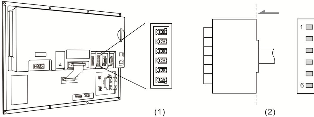
(1) HSI connector on NC controller (Female); (2) HSI connector (Male)
