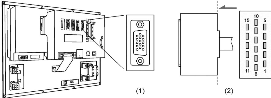
(1) RS-485 connector on NC controller (Female); (2) RS-485 connector (Male)
