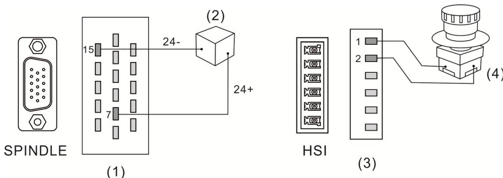
(1) & (3) EMG connector (Female); (2) Power supply; (4) Emergency stop button
