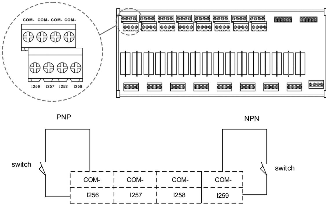
Wiring example: The proximity switch of NPN two-wire system
