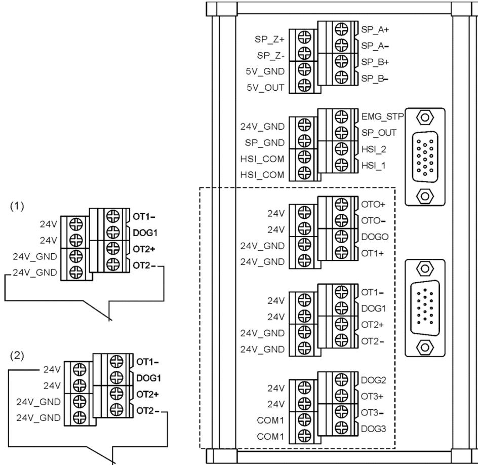
(1) DI input when COM1 connects to 0 V; (2) DI input when COM1 connects to +24 Vdc.
