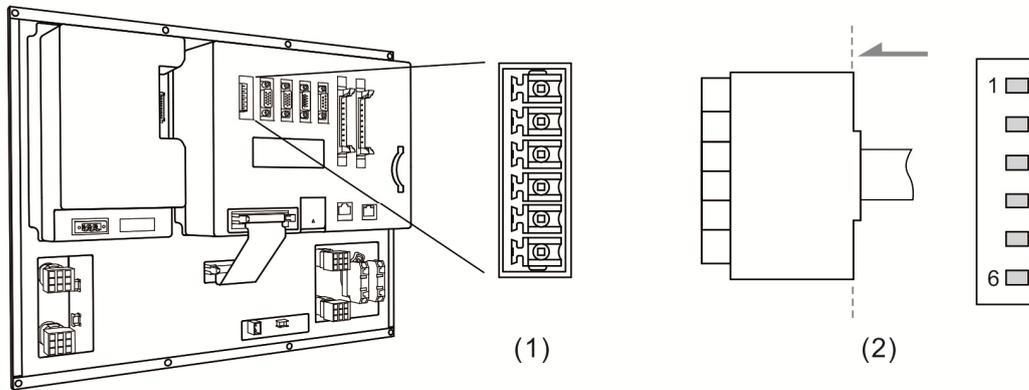
(1) Remote I/O connector on NC controller (Female); (2) Remote I/O connector on the module (Male)
