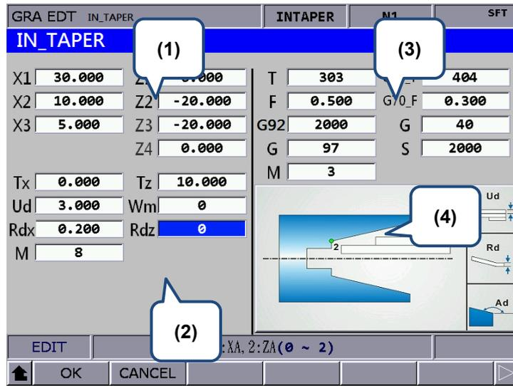
(1) Input the coordinates of each step point (Fields with blue texts can be left blank and it means the point does not exist.)
