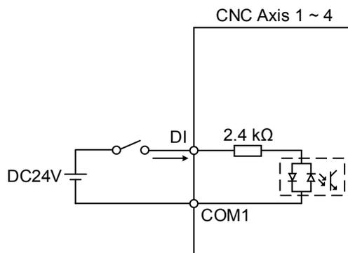
Wiring for Conversion Card (NC-EXM-S01) which connects to AXIS 1 ~ 4 Connector
