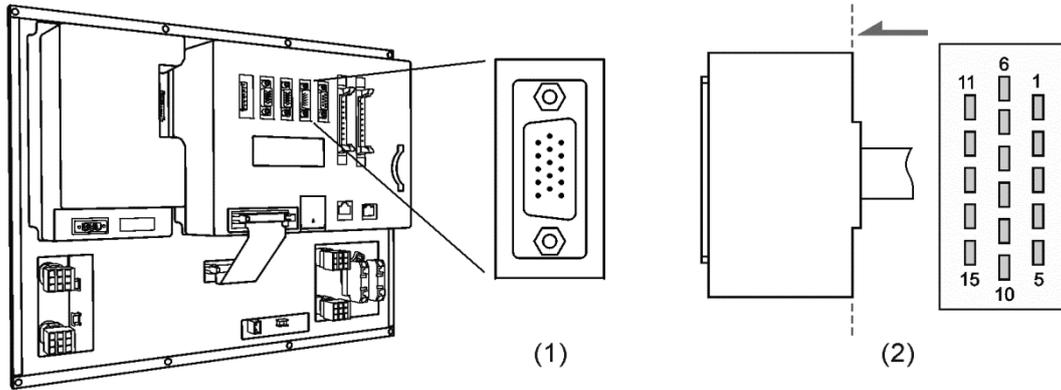
(1) AXIS1 ~ 4 connector on NC controller (Female); (2) AXIS1 ~ 4 connector (Male)
