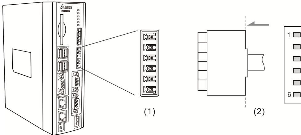
(1) HSI connector on NC controller (Female); (2) HSI connector (Male)
