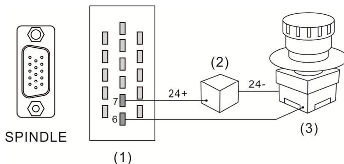
(1) EMG connector (Female); (2) Power supply; (3) Emergency stop button
