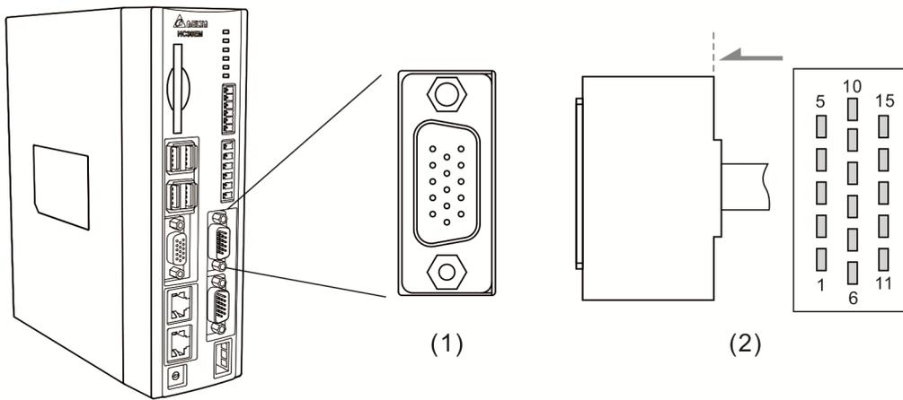
(1) MPG connector on NC controller (Female); (2) MPG connector (Male)
