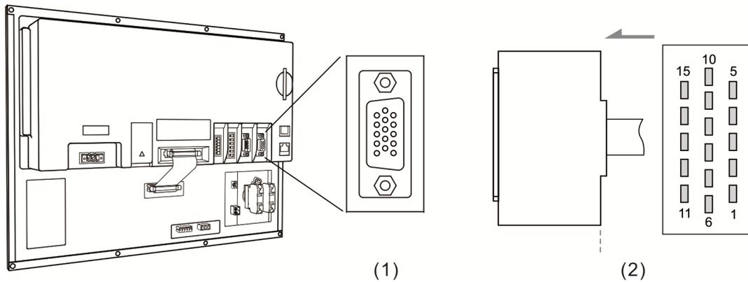
(1) MPG connector on NC controller (Female); (2) MPG connector (Male)
