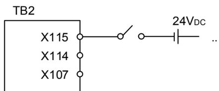
DO wiring, external power supply
