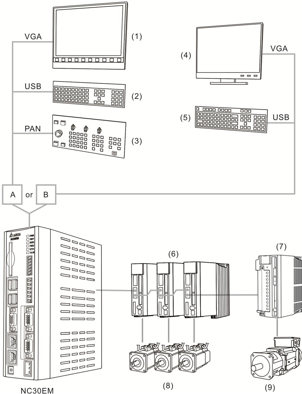
They all connect to (6) ASDA series AC servo drive(s), (7) Spindle servo drive(s) (ASDA-S), (8) ECMA series servo motor(s) and (9) ECMS series spindle motor(s).
