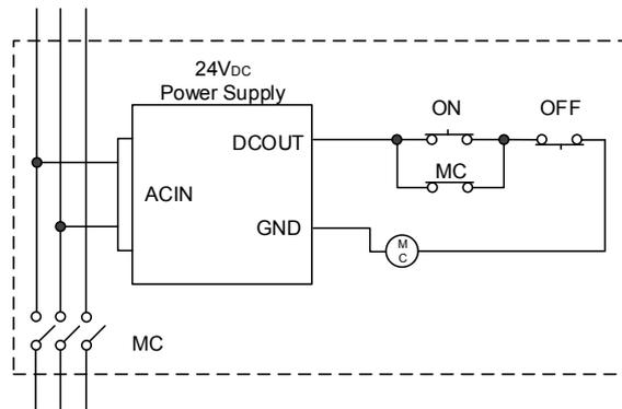
If the Power ON button is pressed, the circuit is closed between PIN ONA1 and ONA2; if the Power OFF button is pressed, the circuit is open between PIN OFFB1 and OFFB2.
