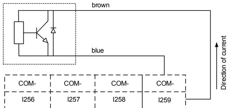
Wiring example: The proximity switch of PNP two-wire system
