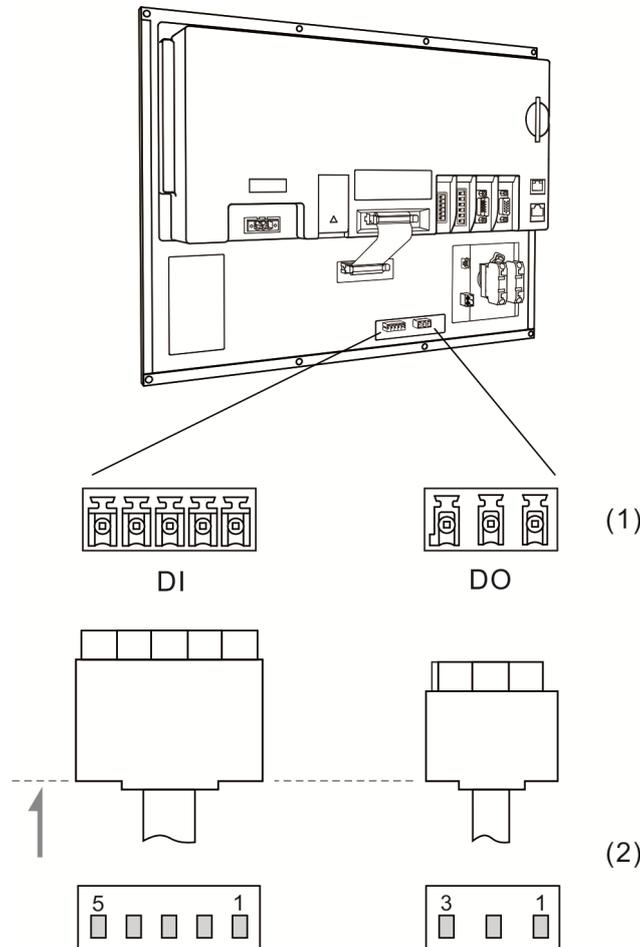
(1) Local I/O connector on NC controller (Female); (2) Local I/O connector (Male)
