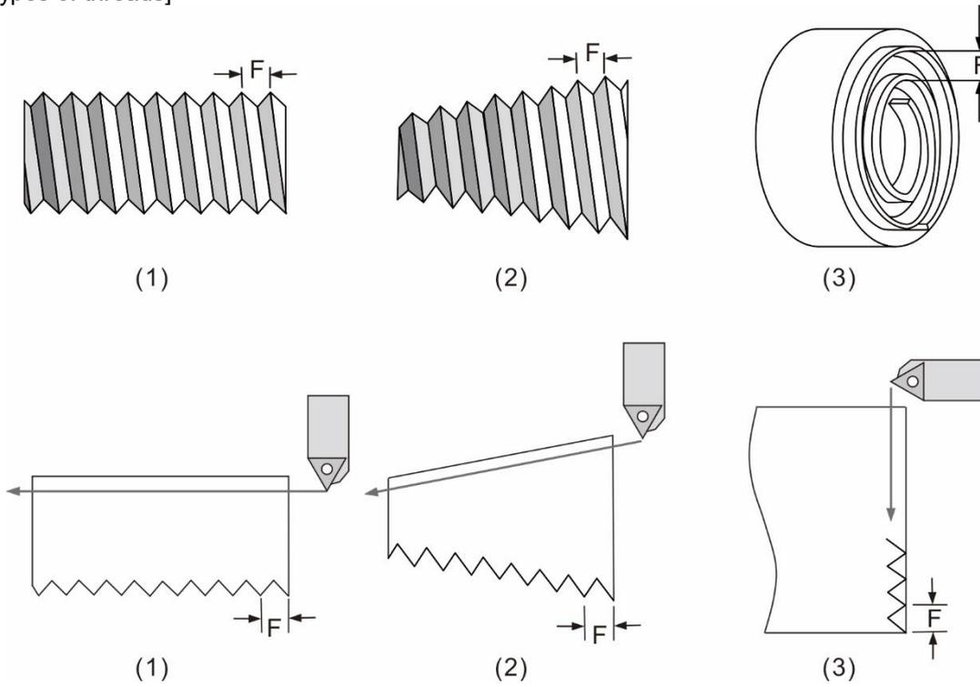
(1) Straight thread; (2) Tapered thread; (3) Scroll thread (face)
