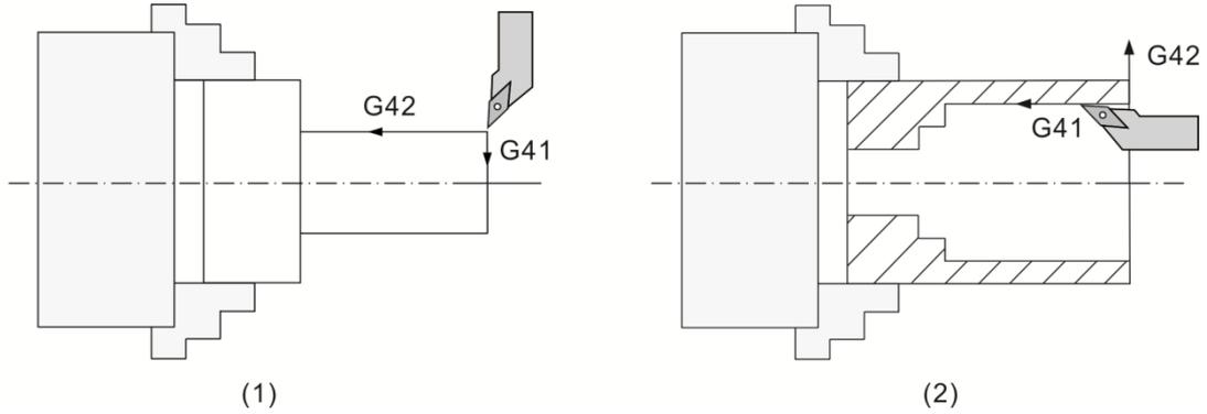
(1) Machining outer diameter and face; (2) Machining inner diameter
