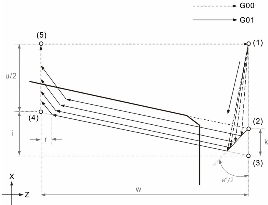
(1) - (5) in the figure represent the tool movement sequence.
