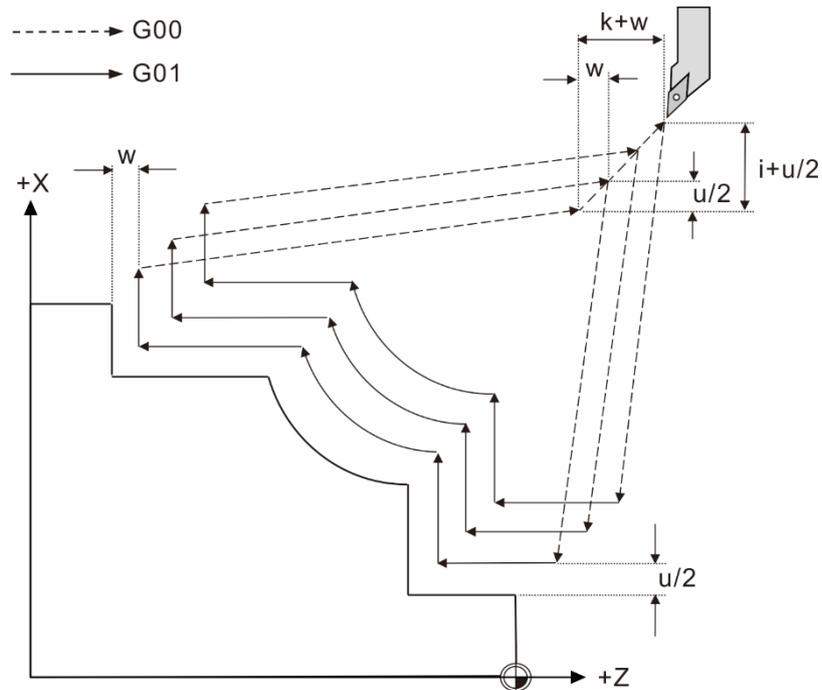
The cutting amount per time: [the total cutting amount of each axis] ÷ [value of cutting times (d-1)]
