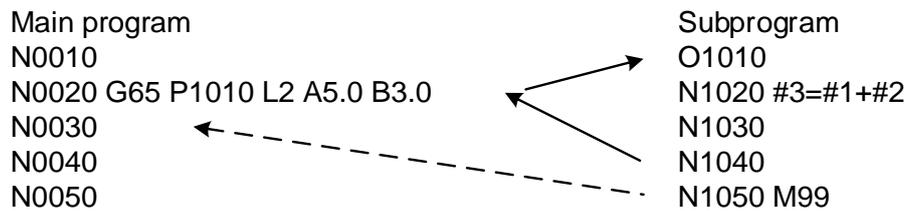
After the macro program is executed, the program returns to the block following G65 command in the main program, which means the block following G65 is executed. See the example above, A5.0 represents variable #1, which value is 5.0. Please refer to the table below.
