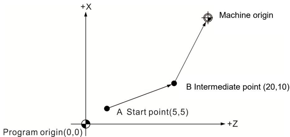
G28 X20. Z10. (Go through the intermediate point B and return to the machine origin.)
