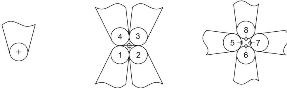
(1) Tool nose No.0 and No.9    (2) Tool nose No. 1 - 4    (3) Tool nose No. 5 - 8
