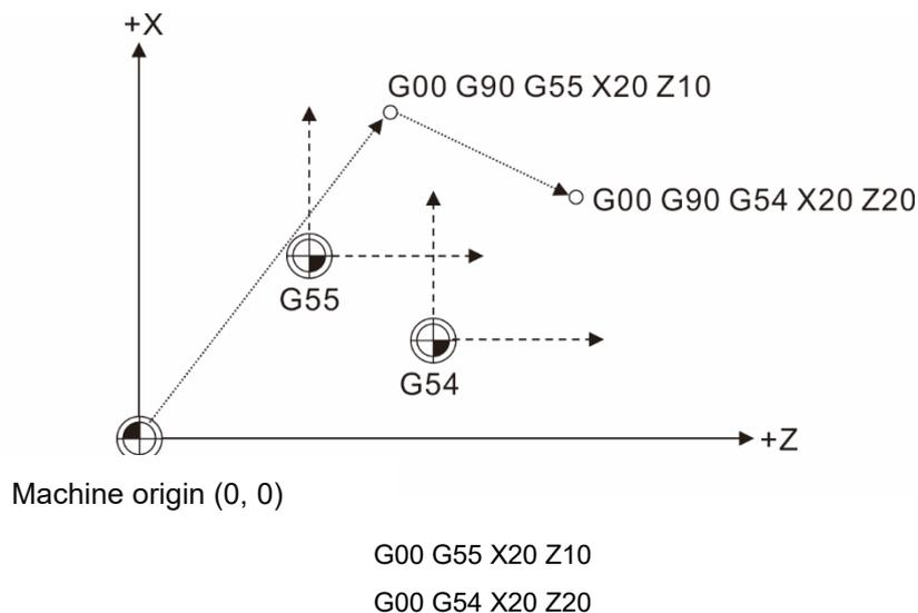
With the workpiece coordinate system settings, you can easily calculate and design the programming path, and create multiple coordinate systems on the work platform for switching among programs. As shown in the figure above, when coordinate origin is changed, you can simply edit the workpiece coordinate data instead of creating another program to carry out machining operations.
