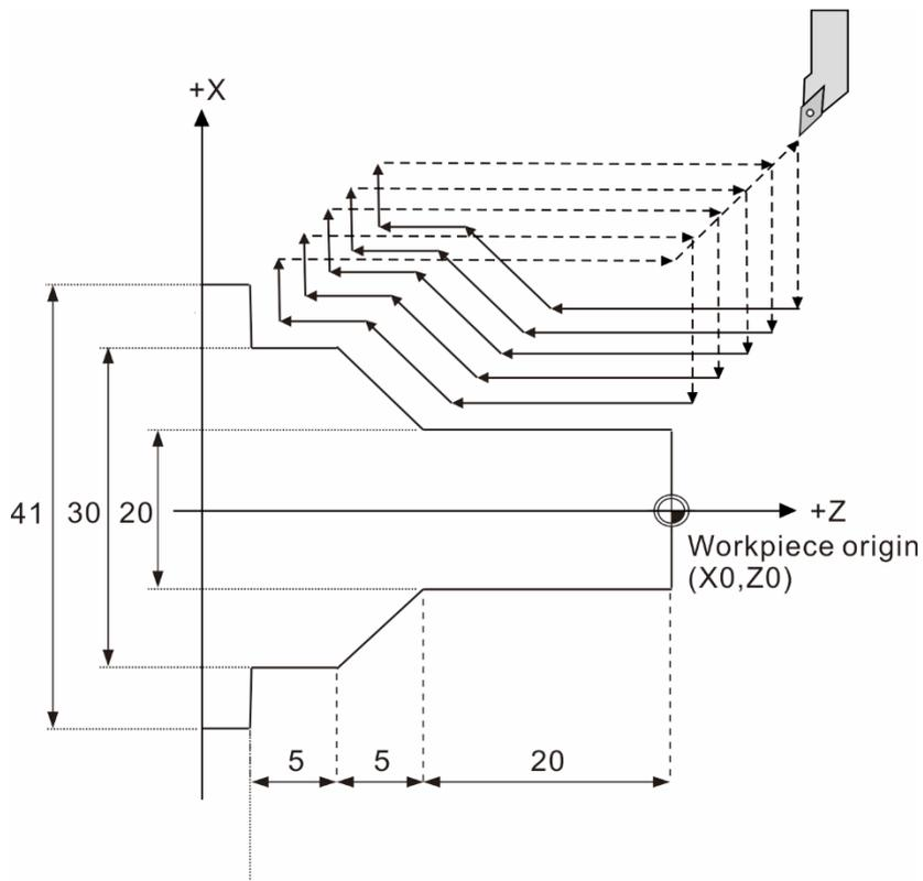
In this program, a bar with diameter 42 mm is used for machining.
