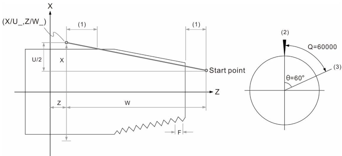
(1) Incorrect leads; (2) Spindle Z-pulse; (3) The point for entering the thread
