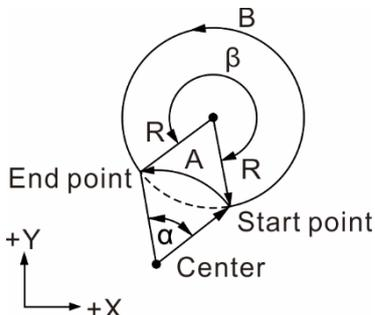
When  $\beta > 180^\circ$ , it means R is a negative value, so arc B is generated.
