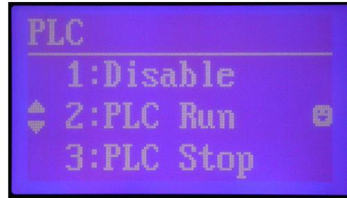
Select PLC run or PLC stop , if the PLC run is chosen then the status of PLC will be running every time when power on
