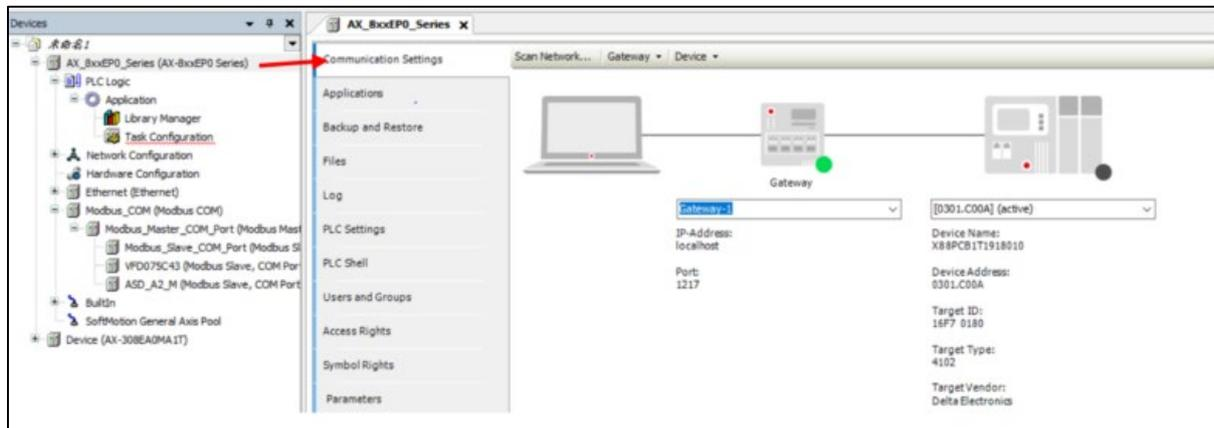
Select a gateway and a target device from the list boxes. The possible selections depend on the entries in the **Manage gateways** and **Manage favorite devices** dialogs (see the **Gateway** menu).
