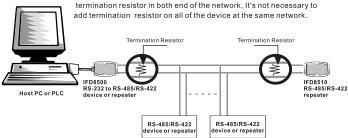
c. If the transmission wire of RS-485 is using twisted pair with 1.2km, We recommend you using resistor with 120 Ohm
