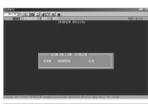
3.Utility will search IFD8520 device from address 0 to 255 with COM1 and 9600bps, You can press any key to stop scan or wait for scan complete
