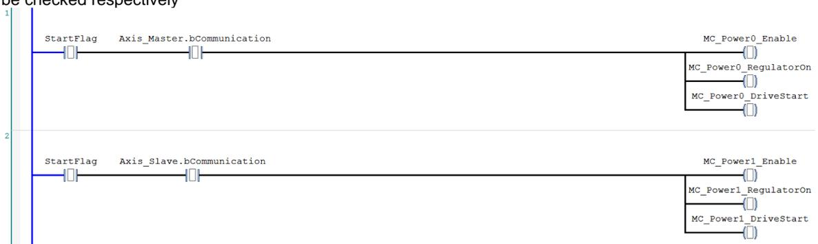
Under normal condition, Servo ON state will be set to master and slave axis.
