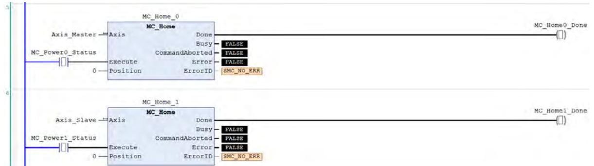
After the homing operation of master axis is completed, execute MC\_MoveVelocity.
