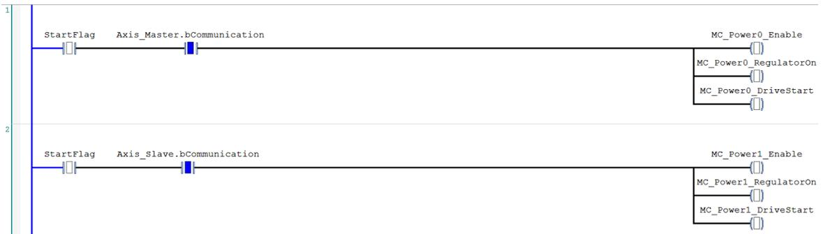
Under normal condition, Servo ON state will be set to master and slave axis.
