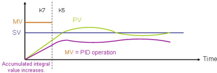
If the control mode becomes the automatic mode (K5), the output value MV changes from the output value set by users to the output value of the PID operation.
