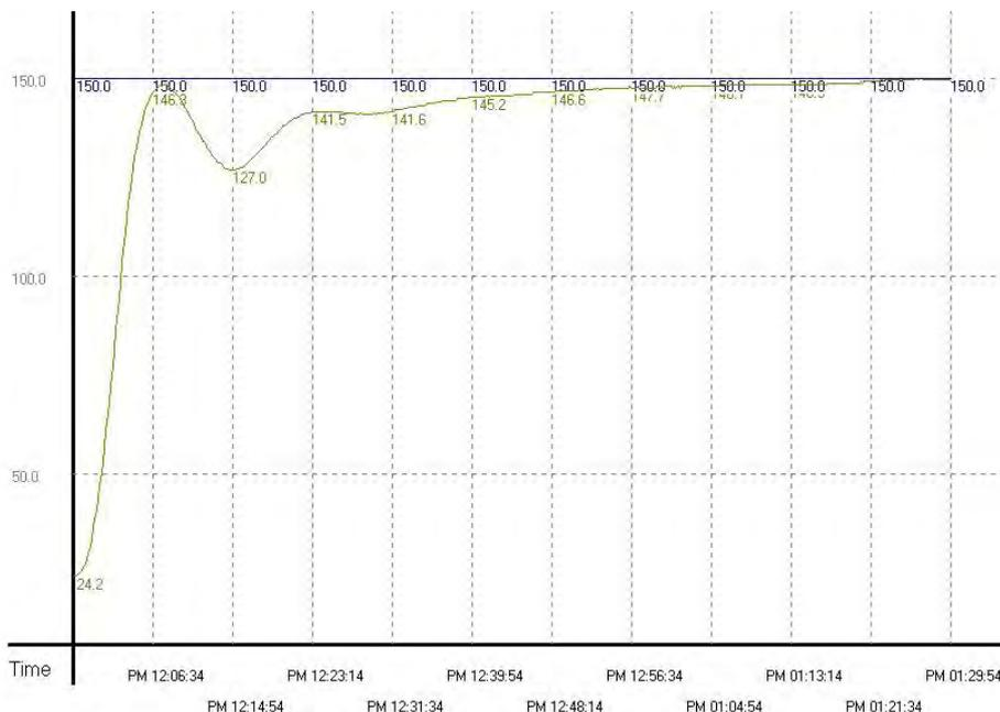
**Example 3:** To speed up the speed to reach the target temperature, we correct the sampling time as 4 seconds (D12 = K40, D30 = K4,000). The results are shown in the diagram below.
