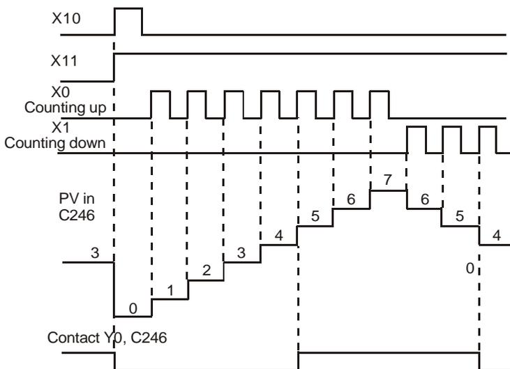
5. The counting modes (normal frequency or double frequency) of C246 (HHSC0) in EH2/SV/EH3/SV2 series MPU can be set up by D1225. The default setting is double frequency mode.
