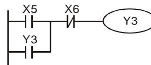
When the circuit is first connected to the power, though X6 is On, X5 is Off, so Y3 will be Off. After X5 is pressed, Y3 will be On. Once Y3 is On, even X5 is released (Off), Y3 can still keep its action because of the draw back (i.e. the self-retained circuit). The actions are illustrated in the table below.
