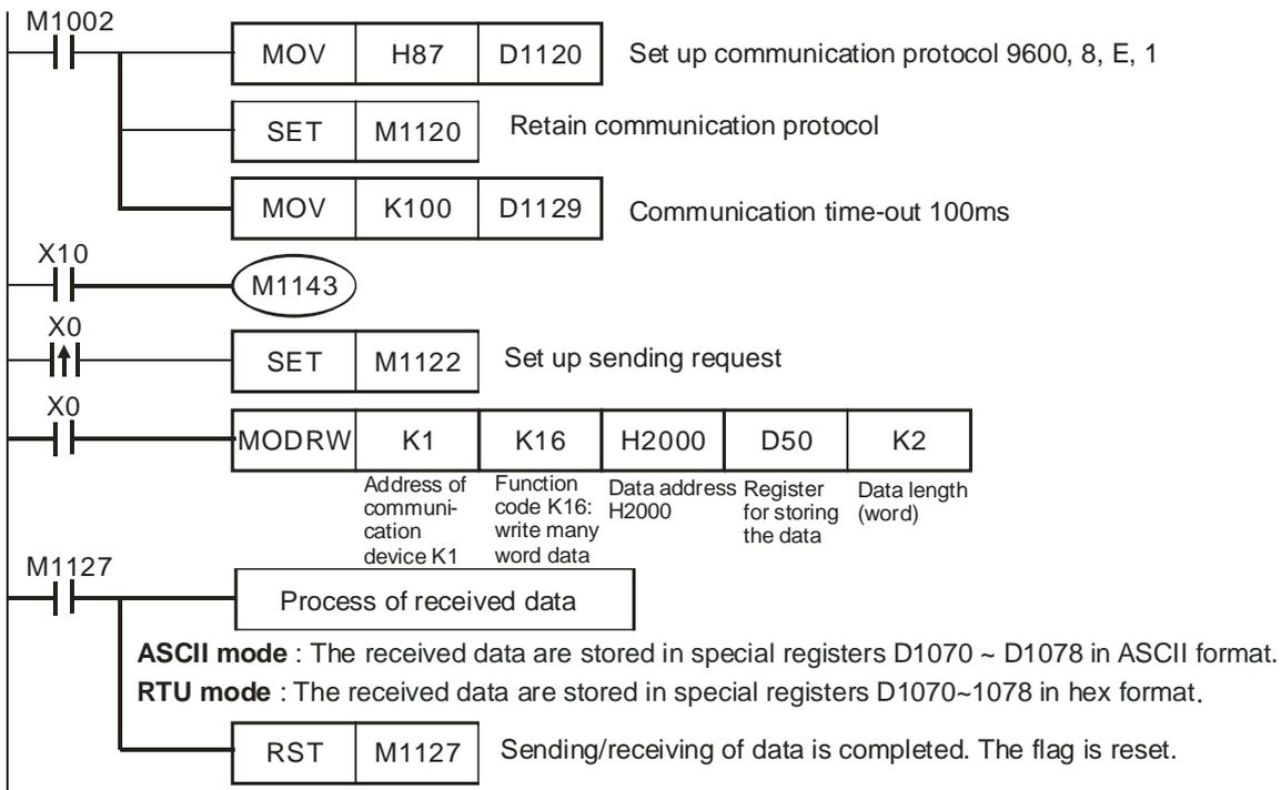
8. ASCII Mode: When PLC is connected to VFD-S AC motor drive.
