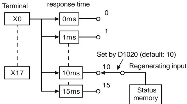
7. If the following programs are executed during the program, the response time of X0 ~ X7 will be set to 0ms. The fastest response time of input terminals is 50μs due to that all terminals are connected with RC filter loop.
