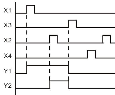
X1 and X3 enables and disables Y1; X2 and X4 enables and disables Y2, and all are latched. Due to that the normally open contact of Y1 is connected to the circuit of Y2 in series, Y1 becomes an AND condition for Y2. Therefore, only when Y1 is enabled can Y2 be enabled.
