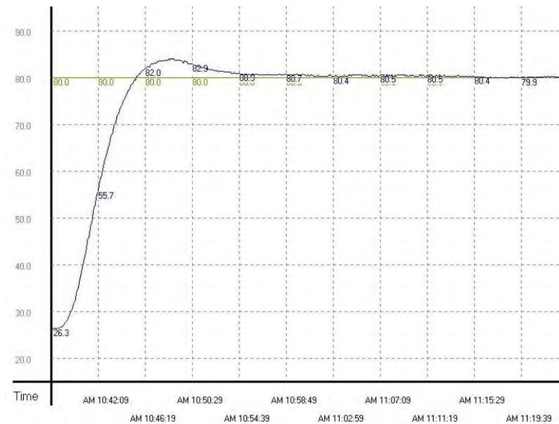
From the figure above, we can see that the temperature control after auto-tuning is working fine and we use only approximately 20 minutes for the control. Next, we modify the target temperature from 80°C to 100°C and obtain the result below.
