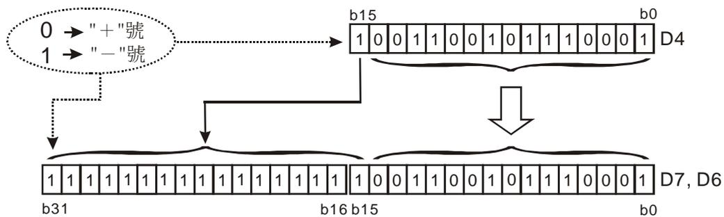
In the example, b15 of D4 is sent to b15 ~ b31 of (D7, D6) as a negative value (same as it is in D4).
