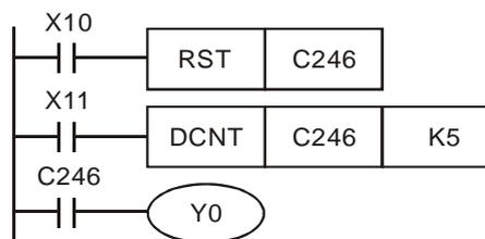
1. When X10 is On, RST instruction will be executed. The PV in C246 will be cleared to "0" and the output contact will be reset to be Off.
