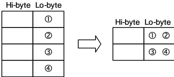
K7: When n = 4, transform 8-bit ASCII data (lower 4 bits, higher 4 bits) into HEX data in the following rule:
