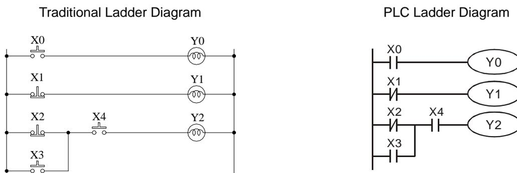
Row 1: Using a normally open (NO) switch X0 (“A” switch or “A” contact). When X0 is not pressed, the contact
