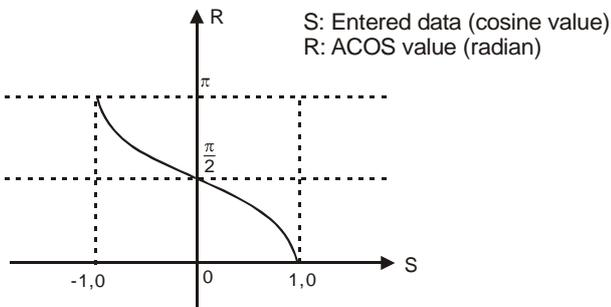
4. The decimal floating point of the COS value designated by **S** should be within -1.0 ~ +1.0. If the value falls without the range, M1067 and M1068 will be On without performing any action.
