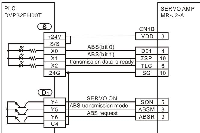
8. **D<sub>2</sub>** will occupy 2 consecutive devices **D<sub>2</sub>** and **D<sub>2</sub> + 1**. **D<sub>2</sub>** is the lower 16 bits and **D<sub>2</sub> + 1** is the higher 16 bits. The absolute position data should be written into the present value registers (D1337, D1336) of CH0 pulse (Y0, Y1)
