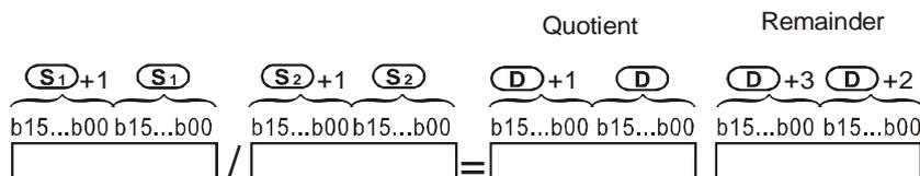
When D serves as a bit device, it can designate K1 ~ K8 and construct a 32-bit result, occupying consecutive 2
