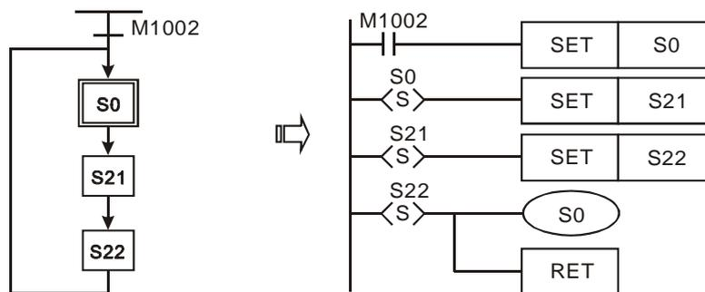
8. RET instruction: Placed after the completed step ladder diagram.
