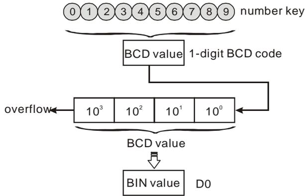
2. As shown in the timing chart below, the 4 points X5, X3, X0, and X1 connected to the keys are entered in order and you can obtain the result 5,301. Store the result in D0. 9,999 is the maximum value allowed to stored in D0. Once the value exceeds 4 digits, the highest digit will overflow.
