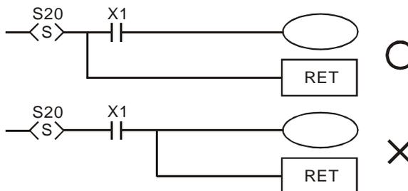
See step ladder instructions [STL], [RET] in Ch. 4 for the structure of the ladder diagram.
