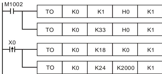
1. Write H0 to CR#1 of analog input module No. 0 and set CH1 as mode 0 (voltage input: -10V ~ +10V).
