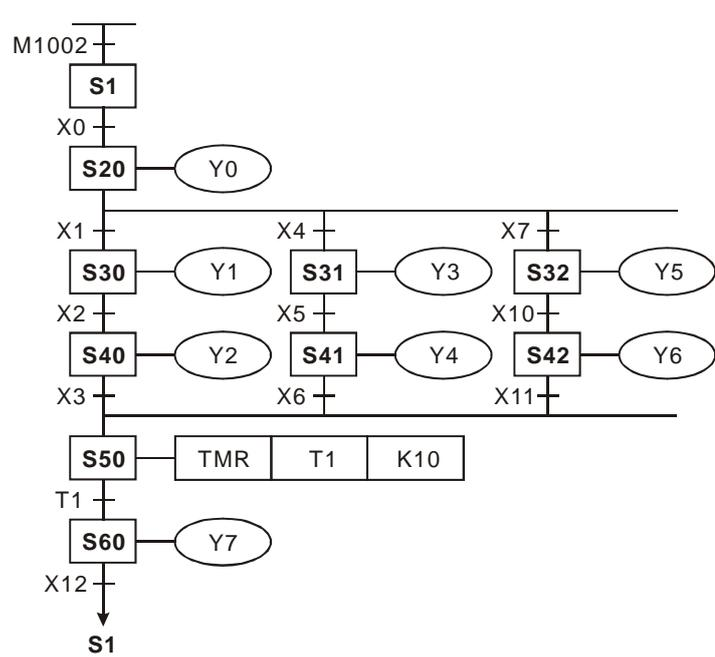
Examples of simultaneous divergence & simultaneous convergence:
