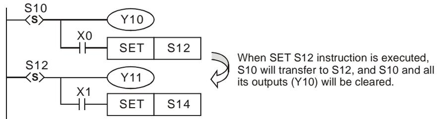
If M1014 is used, and it is On, the transfer of the steps will be prohibited, and the states of the steps remain unchanged.
