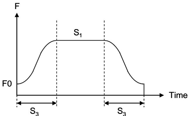
3. The acceleration/deceleration of EH/EH2/SV/EH3/SV2 series MPU is based on the number of pulses. If the output cannot reach the maximum acceleration frequency within the acceleration/deceleration time offered, the instruction will automatically adjust the acceleration/deceleration time and the maximum frequency.
