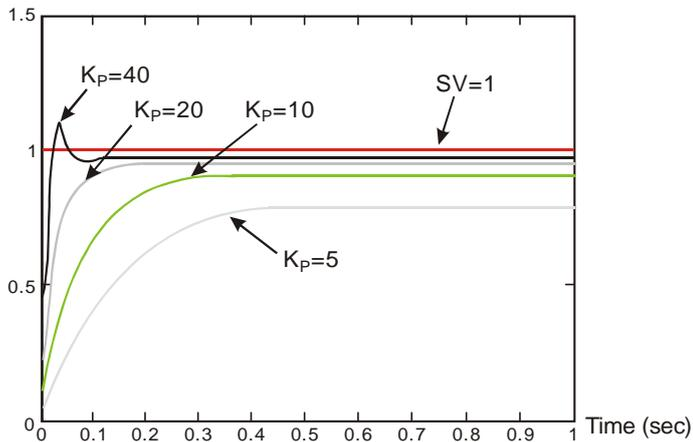
**Step 2:** From the figure, we can see that when  $K_P = 40$ , there will be over-reaction, so we will not select it. When  $K_P = 20$ , the PV reaction curve will be close to SV and there will not be over-reaction, but due to its fast start-up with big transient MV, we will consider to put it aside. When  $K_P = 10$ , the PV reaction curve will get close to SV value more smoothly, so we will use it. Finally when  $K_P = 5$ , we will not consider it due to the slow reaction.
