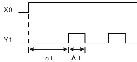
The ladder diagram program controls the On time of coil Y1 by timer T0 and disable timer T0 in the next scan cycle, resulting in the oscillating pulses in the output of Y1. n refers to the decimal set value in the timer and T is the cycle of the clock.
