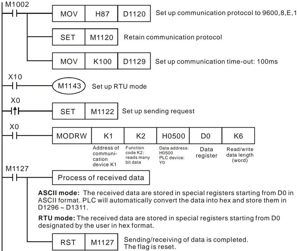
2. ASCII Mode: When PLC1 is connected to PLC2
