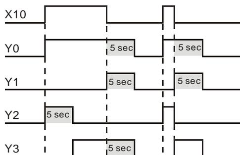
6. Add a b contact of Y3 after X10, and Y1 and Y2 can operate for flashing sequence output. When X10 goes Off, Y0, Y1 and Y3 will be Off and the content in T10 will be reset to 0.
