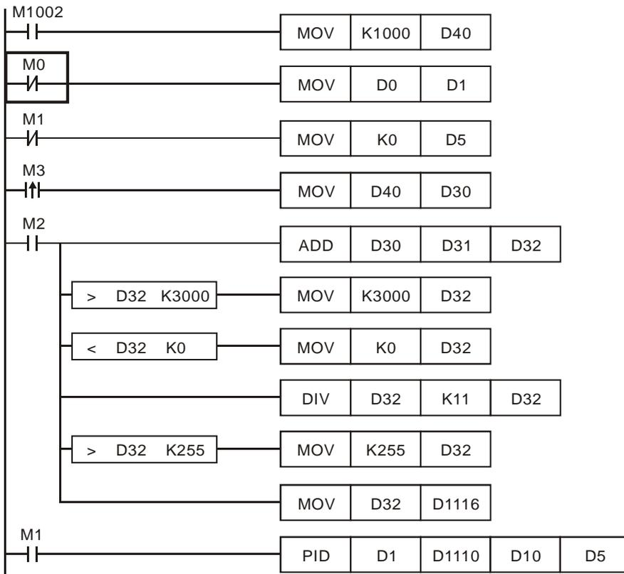
**Application 3** Using auto-tuning on the parameter for the temperature control.
