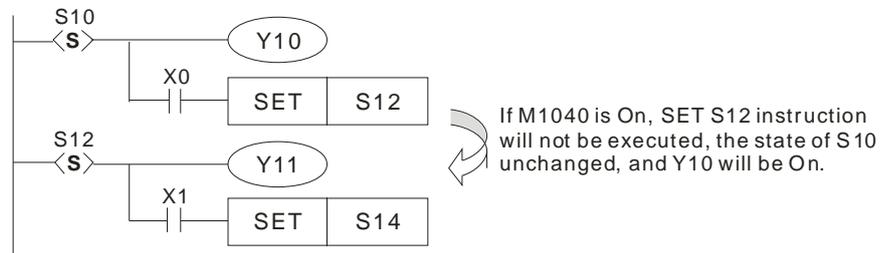
**OUT Sn** Used for returning to the initial step in the same step sequence. Also for jumping up/down to non-adjacent steps in the same sequence, or separating steps in different sequences. After the transition, all output from the previous status will be cleared.
