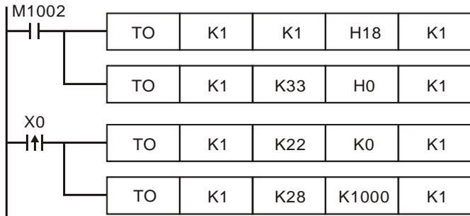
1. Write H18 to CR#1 of analog output module No. 1 and set CH2 as mode 3 (current output: 0mA ~ +20mA).
