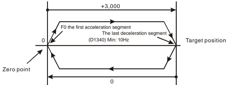
b) Settings of absolute positioning and the acceleration/deceleration speed:
