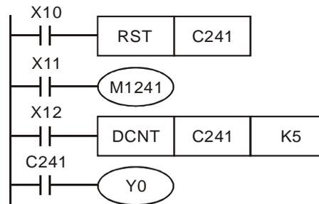
1. X11 drives M1241 to determine whether C241 is an addition or subtraction counter.
