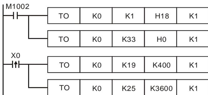
1. Write H18 to CR#1 of analog input module No. 0 and set CH2 as mode 3 (current input: -20mA ~ +20mA).
