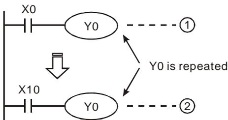
The output of Y0 will be determined by circuit ②, i.e. On/Off of X10 will determine the output status of Y0.
