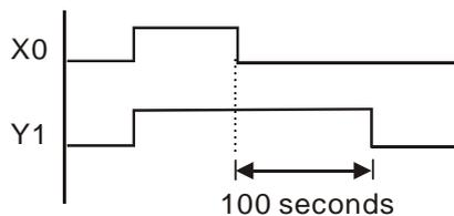
When input X0 is On, due to that its corresponding normally closed contact is Off, time T10 will be Off and the output coil Y1 will be On. T10 will be On and start to count until input X0 is Off. Output coil Y1 will be delayed for 100 seconds ( $K1,000 \times 0.1 \text{ sec} = 100 \text{ secs}$ ) and be Off. See the timing diagram above.
