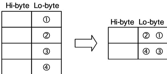
K8: Transform 8-bit GPS data into 32-bit floating point data in the following rule:
