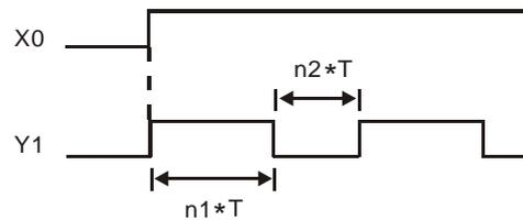
The ladder diagram is an oscillating circuit which makes the indicator flash or enables the buzzer alarms. It uses two timers to control the On/Off time of coil Y1. n1 and n2 refer to the set values in T1 and T2 and T is the cycle of the clock.
