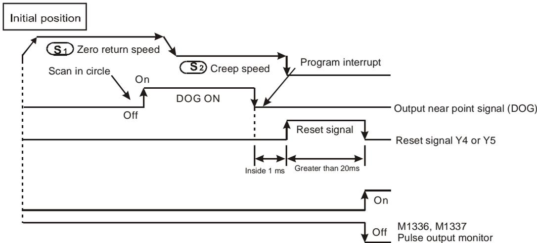
**Note:** The designated devices, X, Y, M, and S, other than the external input devices X10 ~ X17 will be affected by the scan period, 2 times of the scan period at worst.
