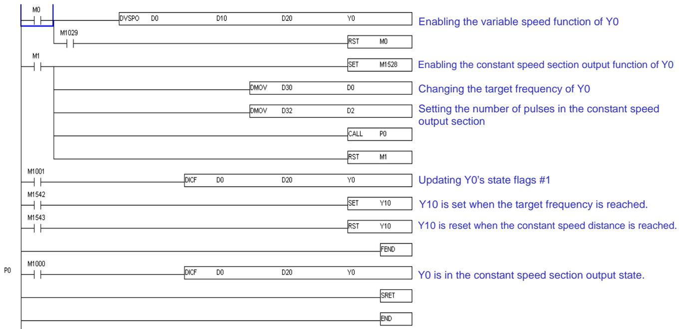
Note 1: If DICF is not enabled, and the constant speed output section is executed, the instruction will constantly check whether the target frequency is reached and whether the output state is complete, and will set the corresponding flags. If the scan time is long, users can insert many lines of DICF instructions, or execute DICF in a time interrupt (do not need to enable the instruction) to update the output state constantly.
