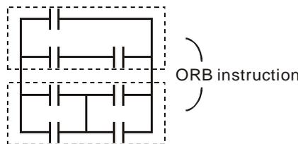
If the ANB and ORB operations are with several blocks, the operation should be performed from up to down or left to right, combining into a block or network.
