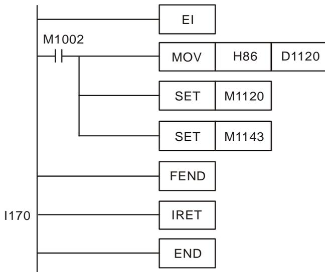
With I170 in the program, when COM2 is in Slave mode and there are communication data coming in, PLC will process the data and respond immediately.
