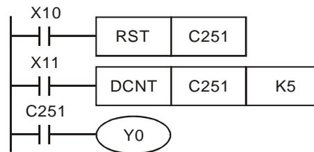
1. When X10 is On, RST instruction will be executed. The PV in C251 will be cleared to "0" and the output contact will be reset to be Off.
