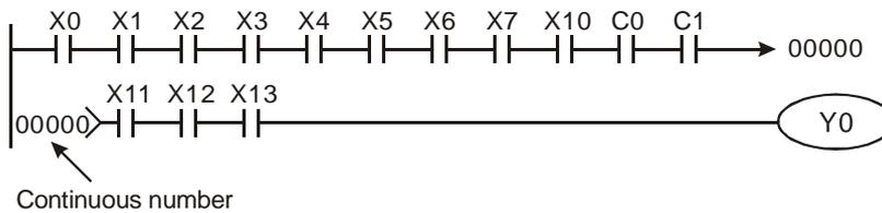
The operation of the ladder diagram program is scanning from top left to bottom right. The coil and the operation frame of the application instruction belong to the output side in the program and are placed in the right if the ladder diagram. Take the figure below for example, we will step by step explain the process of a ladder diagram. The numbers in the black circles indicate the order.
