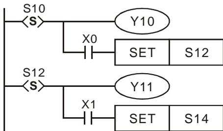
Executing the timing diagram below. After the status of S10 and S12 are transferred (taking place simultaneously), and after a delay of 1 scan time, Y10 will be Off and Y11 will be On. There will not be overlapping outputs.
