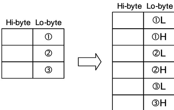
K6: When n = 4, transform 8-bit ASCII data (higher 4 bits, lower 4 bits) into HEX data in the following rule:
