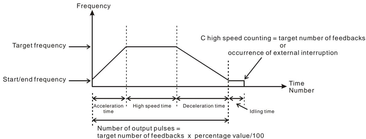
3. How to adjust the time for the completion of the positioning:
