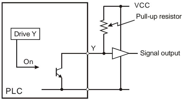
6. Positive logic (negative polarity) output of BCD code
