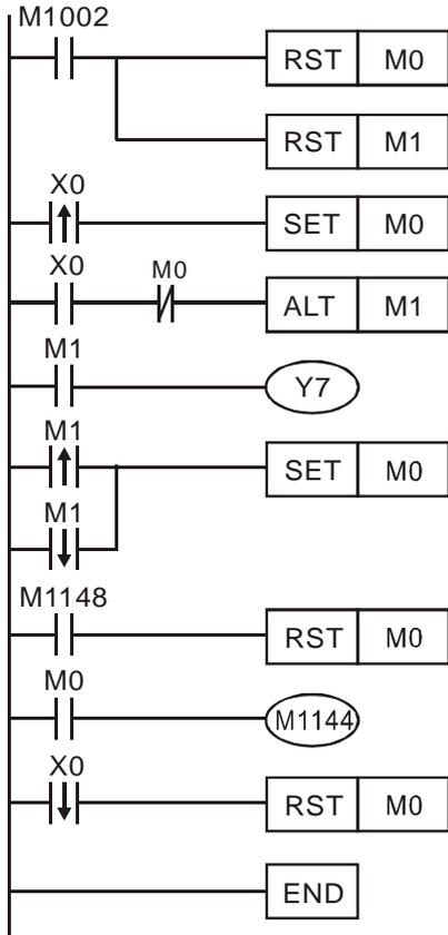
8. Example 4: Program of zero return for 1 acceleration section and 1 deceleration section
