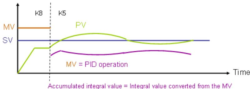
If the control mode becomes the automatic mode (K5), the accumulated integral value will be the integral value converted from the last MV, and the accumulated integral value will be converted into the output value of the PID operation.
