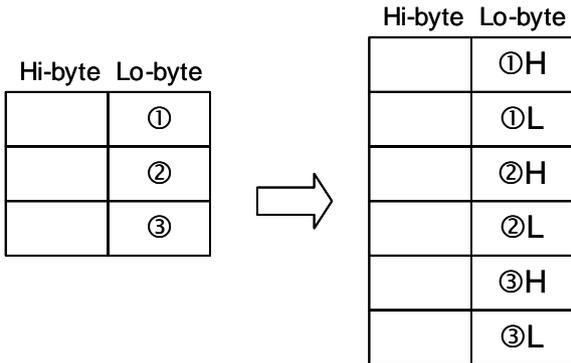
K5: With  $n = 3$ , transform 8-bit HEX data into ASCII data (lower 4 bits, higher 4 bits) in the following rule:
