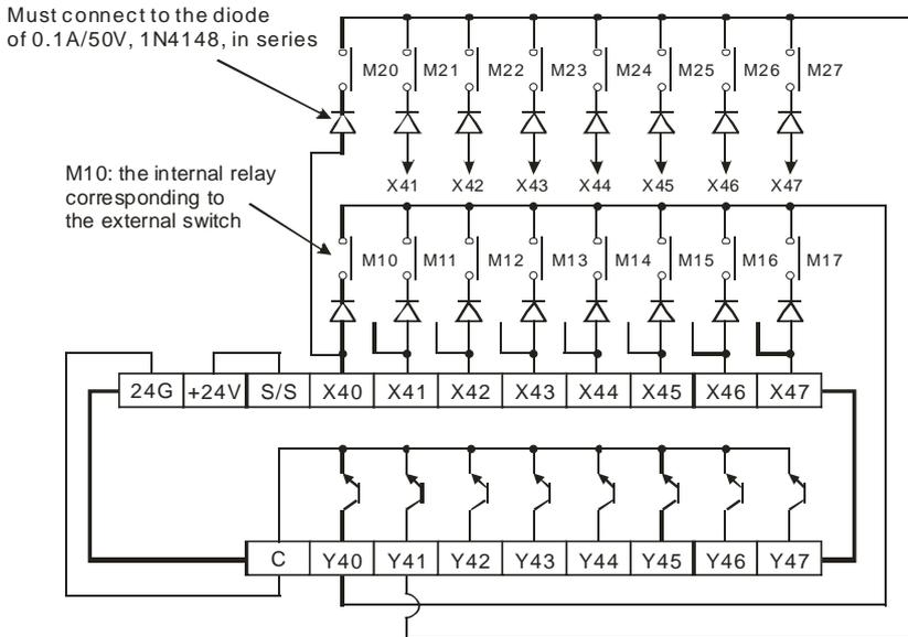
3. See the figure above. The 8 points starting from X40 start to perform a matrix scan from Y40 ~ Y41 (n = 2). **D<sub>2</sub>** designates that the start device No. of the read results is M10, indicating that the first array is read to M10 ~ M17 and the second array is read to M20 ~ M27.
