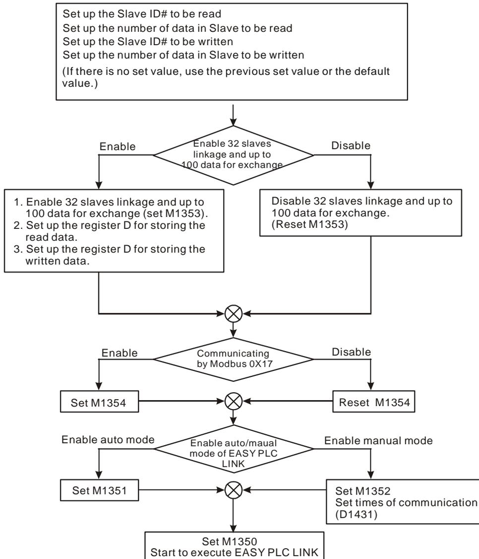
a) Example 1: Enabling 32 slave units linkage and up to 100 data for exchange in PLC LINK by M1353
