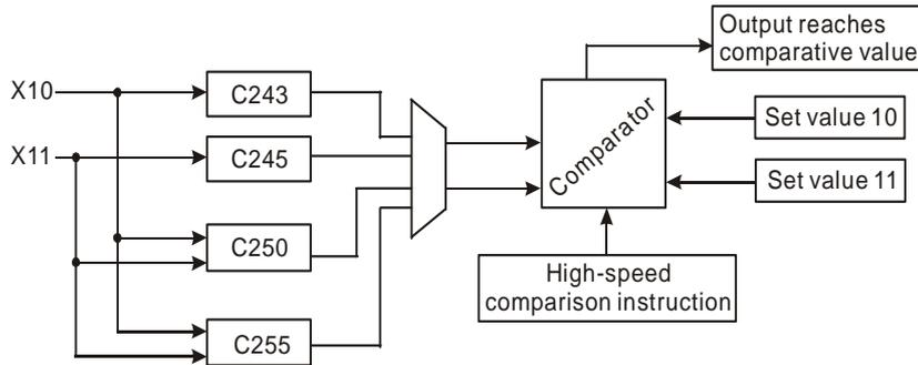
vi) Explanations on high speed counter and high speed comparator:
