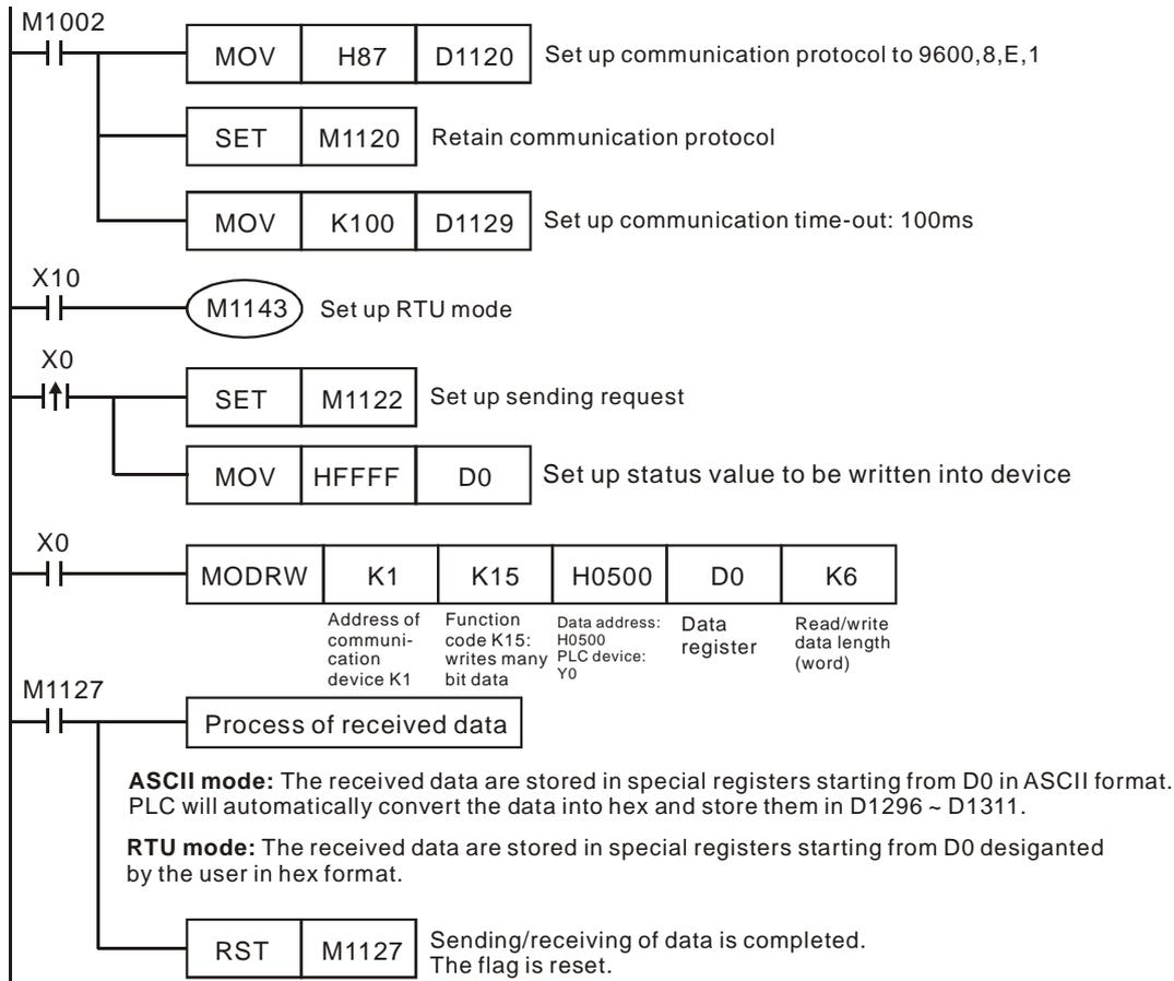
2. ASCII Mode: When PLC1 is connected to PLC2
