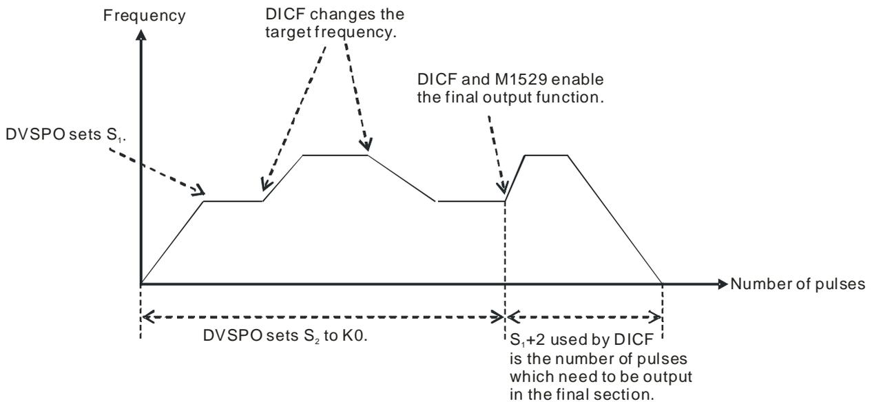
2. The target frequency in the final section is lower than the current output frequency
