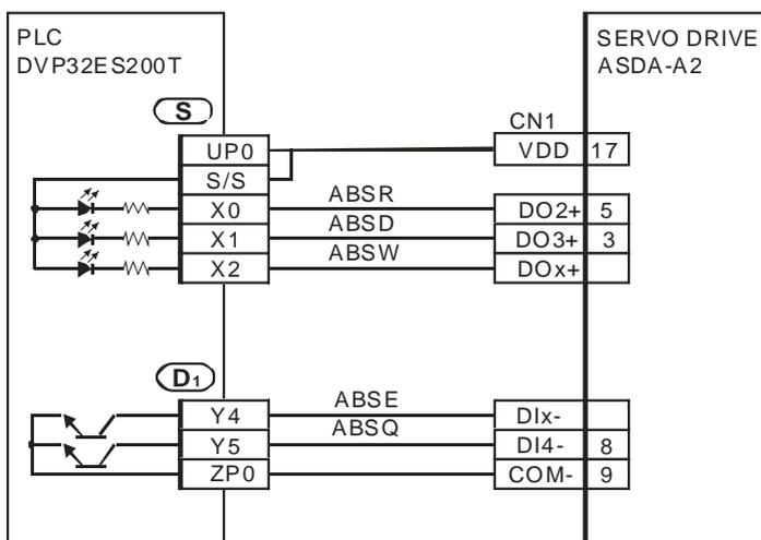
5. **D<sub>2</sub>** will occupy 4 consecutive devices **D<sub>2</sub>**, **D<sub>2</sub> +1**, **D<sub>2</sub> +2**, and **D<sub>2</sub> +3**. The absolute acoordinate system status (P0-50) is stored in **D<sub>2</sub>**, the encoder absolute position (multiturn) (P0-51) is stored in **D<sub>2</sub> +1**. The lower 16 bits of
