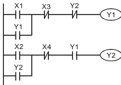
If we serially connect the normally closed contact of Y2 in example 5 to the circuit of Y1 as an AND condition for Y1 (as the diagram in the left hand side), the circuit can not only make Y1 as the condition for Y2, but also allow the stop of Y1 after Y2 is enabled. Therefore, we can make Y1 and Y2 execute exactly the sequential control.
