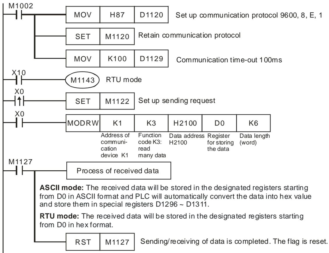
9. ASCII Mode: When PLC is connected to VFD-S AC motor drive.
