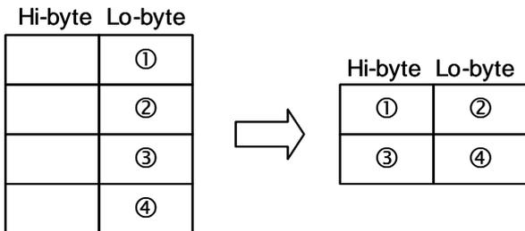
K1: With n = 4, transform 8-bit data into 16-bit data (Lo-byte, Hi-byte) in the following rule:
