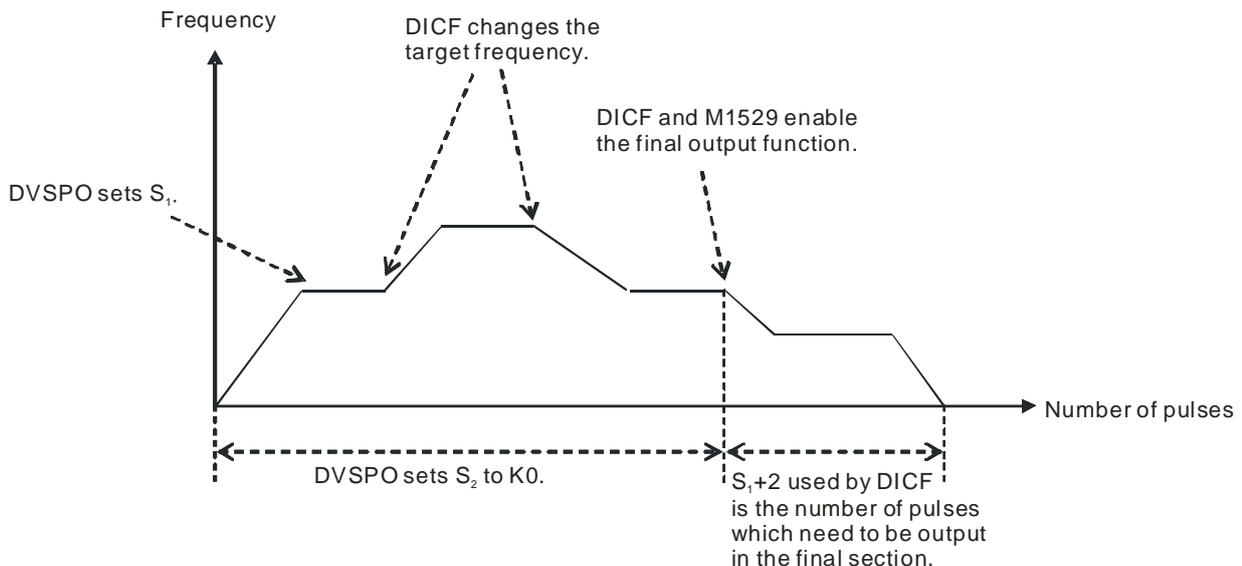
Note 1: Although there will be no limit on the number of output pulses if  $S_2$  is K0, the number of pulses in the final section will be the target number of pulses in the final section after the final output section is enabled, and
