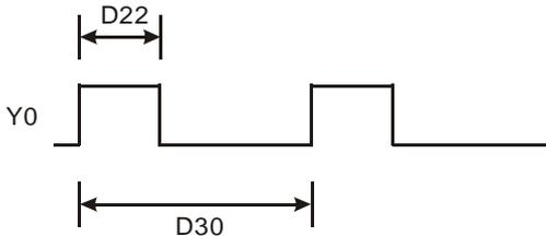
Assume parameter settings: D10 = K1,500 (target temperature), D12 = K60 (sampling time: 6 secs.), D13 = K8 (bit3=1), D30 = K6,000 (=D12\*100)
