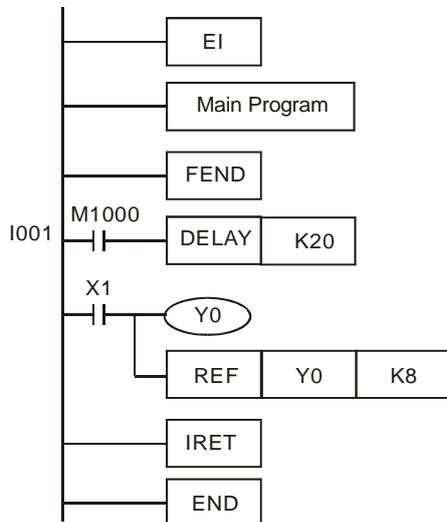
If X0 is turned from Off to On, the external interruption will be generated. Owing to the fact that M1148 is ON, DELAY in the interrupt subroutine will be execute for 100 ms before the next step (X1 = On and Y0 = On) is executed.
