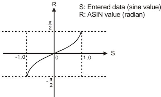
4. The decimal floating point of the SIN value designated by **S** should be within -1.0 ~ +1.0. If the value falls without the range, M1067 and M1068 will be On without performing any action.
