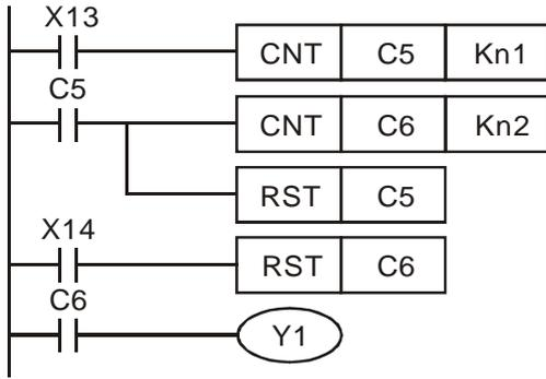
The counting range of a 16-bit counter is 0 ~ 32,767. As the circuit in the left hand side, using two counters can increase the counting range to  $n_1 * n_2$ . When the counting of counter C5 reaches  $n_1$ , C6 will start to count for one time and reset for counting the pulses from X13. When the counting of counter C6 reaches  $n_2$ , the pulses from input X13 will be  $n_1 * n_2$ .
