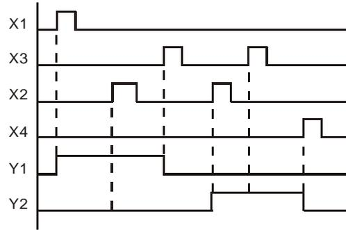
Which of the X1 and X2 is first enabled decides either the corresponding output Y1 or Y2 will be enabled first. Either Y1 or Y2 will be enabled at a time, i.e. Y1 and Y2 will not be enabled at the same time (the interlock). Even X1 and X2 are enabled at the same time, Y1 and Y2 will not be enabled at the same time due to that the ladder diagram program is scanned from up to down. In this ladder diagram, Y1 will be enabled first.
