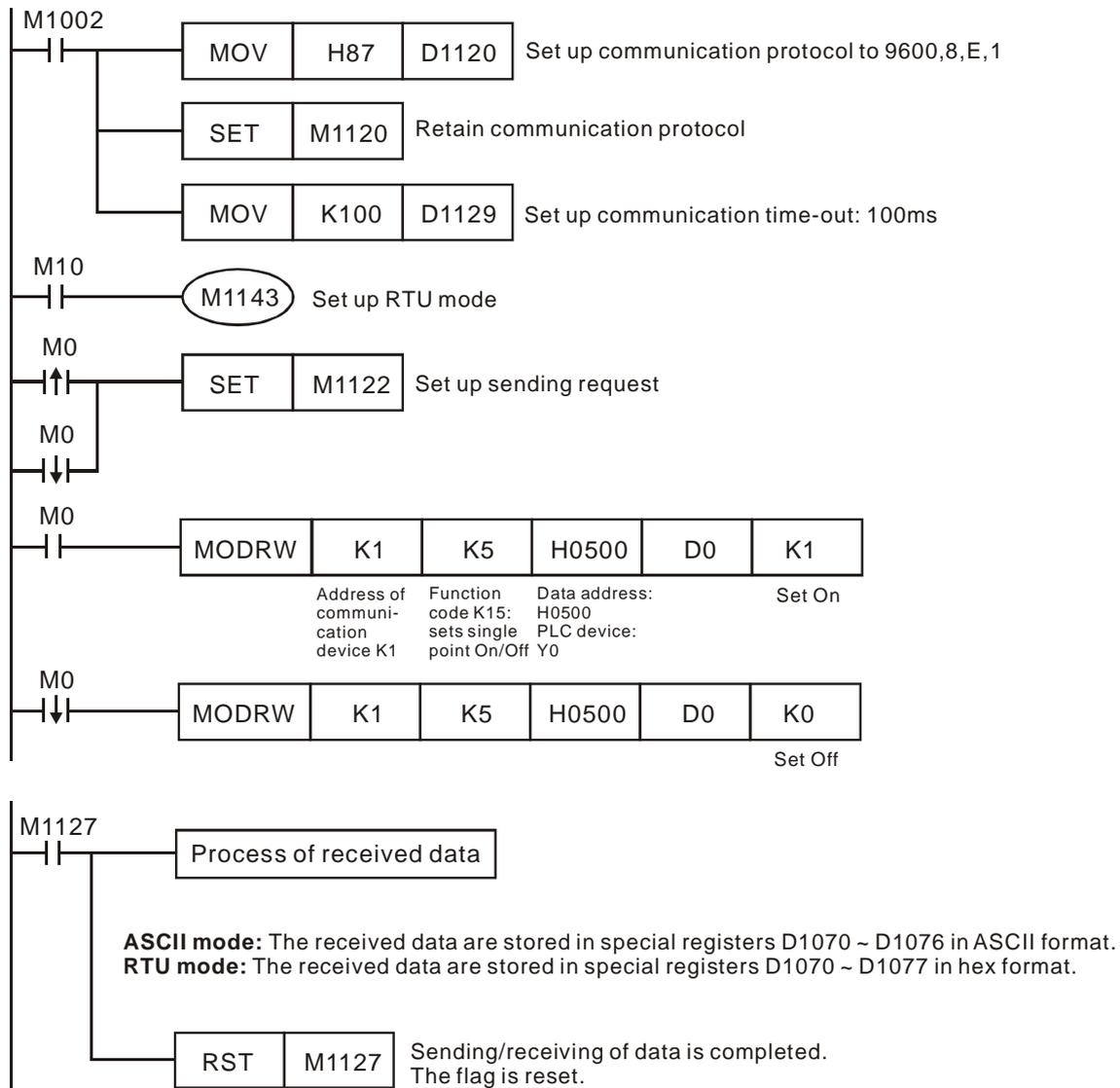
2. ASCII Mode: When PLC1 is connected to PLC2
