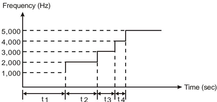
From the conditions above, we can obtain the number of acceleration/deceleration sections is  $(5K - 1K)/1K = 4$  and the number of output pulses in each section is  $40/4 = 10$ . Therefore, in the diagram,  $t1 = (1/1K) \times 10 = 10\text{ms}$ ,  $t2 = (1/2K) \times 10 = 5\text{ms}$ ,  $t3 = (1/3K) \times 10 = 3.33\text{ms}$ ,  $t4 = (1/4K) \times 10 = 2.5\text{ms}$ .
