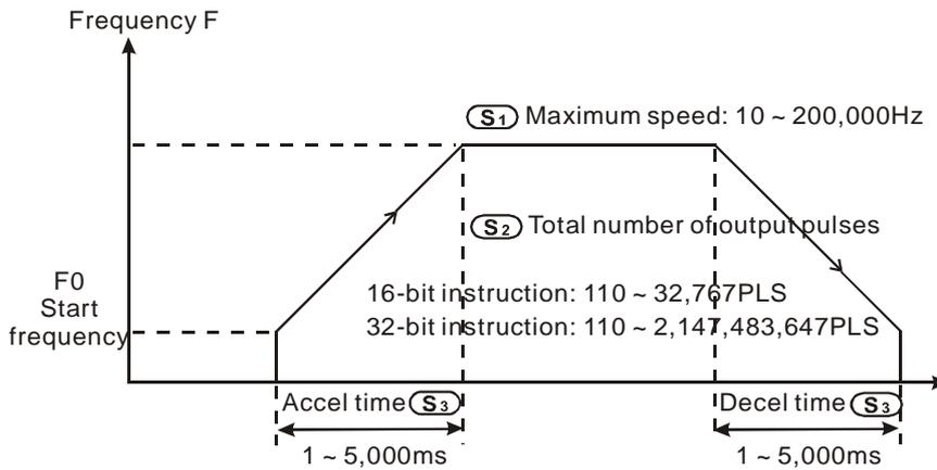
When M1257 is On, the acceleration/deceleration slope is an S curve, as shown below.
