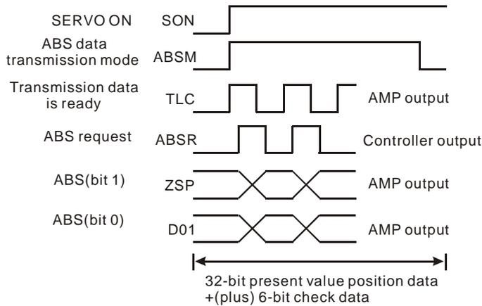
3. This instruction is applicable to the Servo motor equipped with absolute positioning function, e.g. Mitsubishi MR-J2-A Servo drive.
