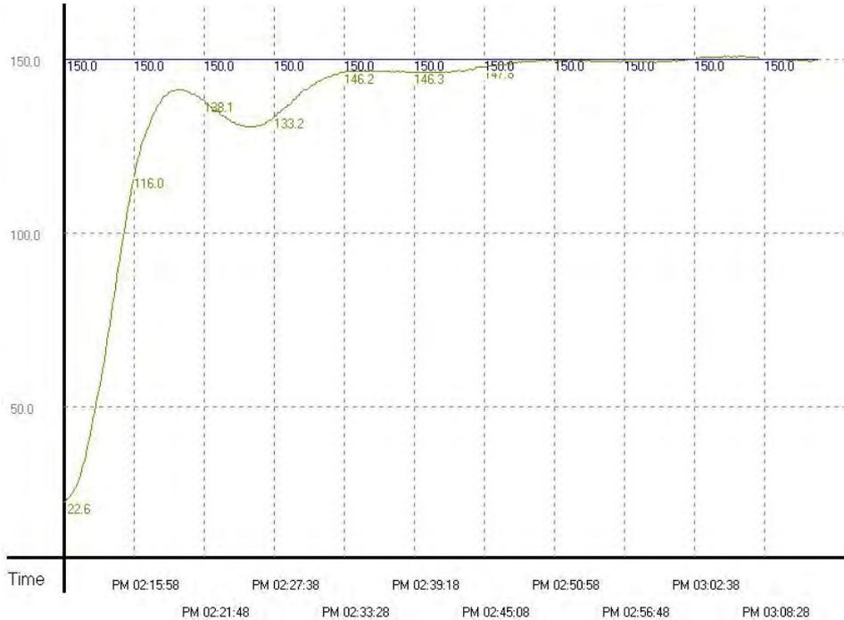
**Example 4:** To see if we can reach the target temperature faster, we modify the sampling time from example 3 into 2 seconds (D12 = K20, D30 = K2,000). The results are shown in the diagram below.
