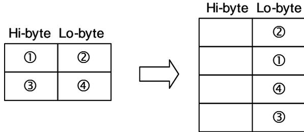
K4: With  $n = 3$ , transform 8-bit HEX data into ASCII data (higher 4 bits, lower 4 bits) in the following rule:
