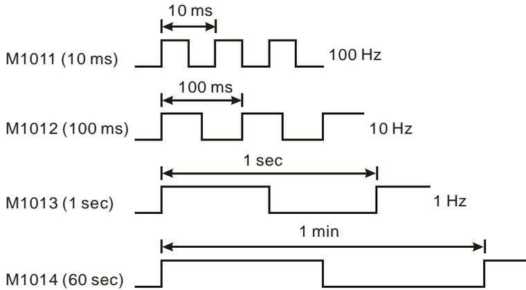
2. The clock pulses also start when PLC is in STOP status. The activation timing of clock pulses and that of RUN will not happen synchronously.
