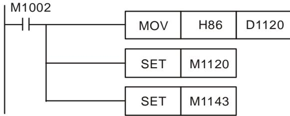
3. EH2/SV/EH3/SV2 series MPU supports the generation of interruption I170 when the data receiving is completed in Slave mode.
