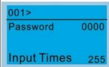
If the WPLSoft editor is installed and uses password, enter the password to save the file to the keypad.
