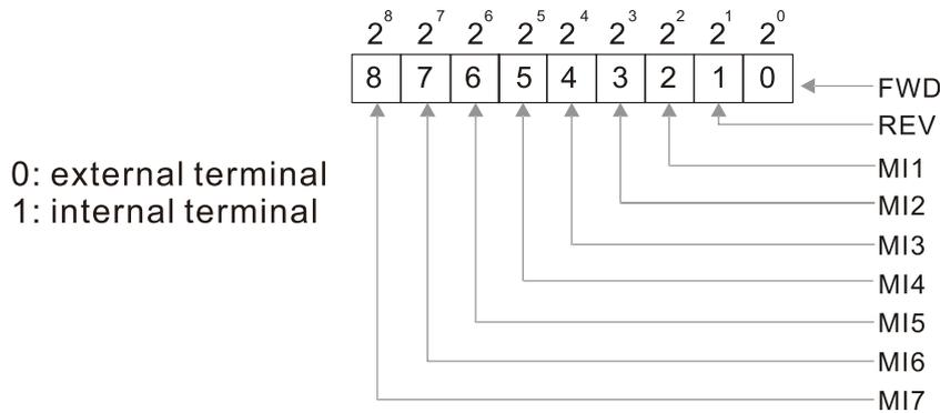
Setting method: convert the binary 12bit number to hexadecimal number for input.
