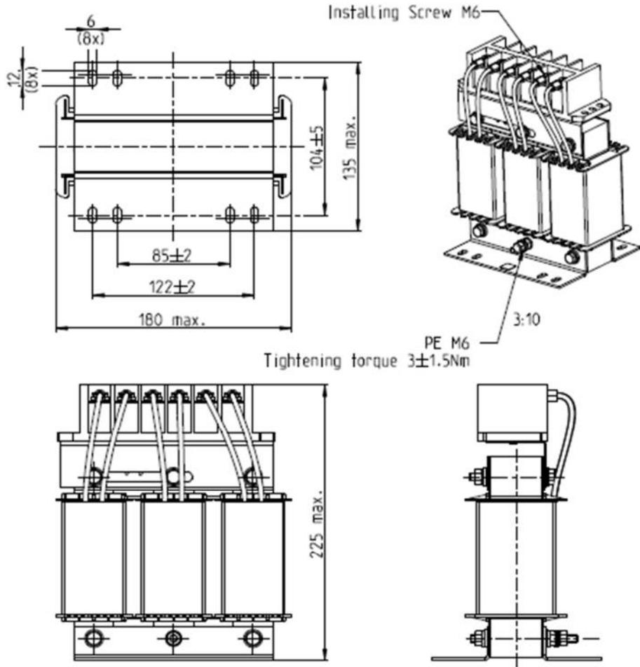
Tightening torque  $3 \pm 1.5 \text{ Nm}$
