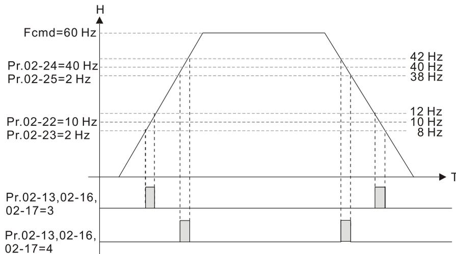
**02-34** Output Frequency Setting for Multi-function Output Terminal
