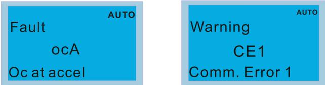
1. Press the STOP / RESET key to reset the fault code. If there is no response, contact your local distributor or return the unit to the factory. To view the fault DC bus voltage, output current and output voltage, press MENU and then choose 6: Fault Record.
