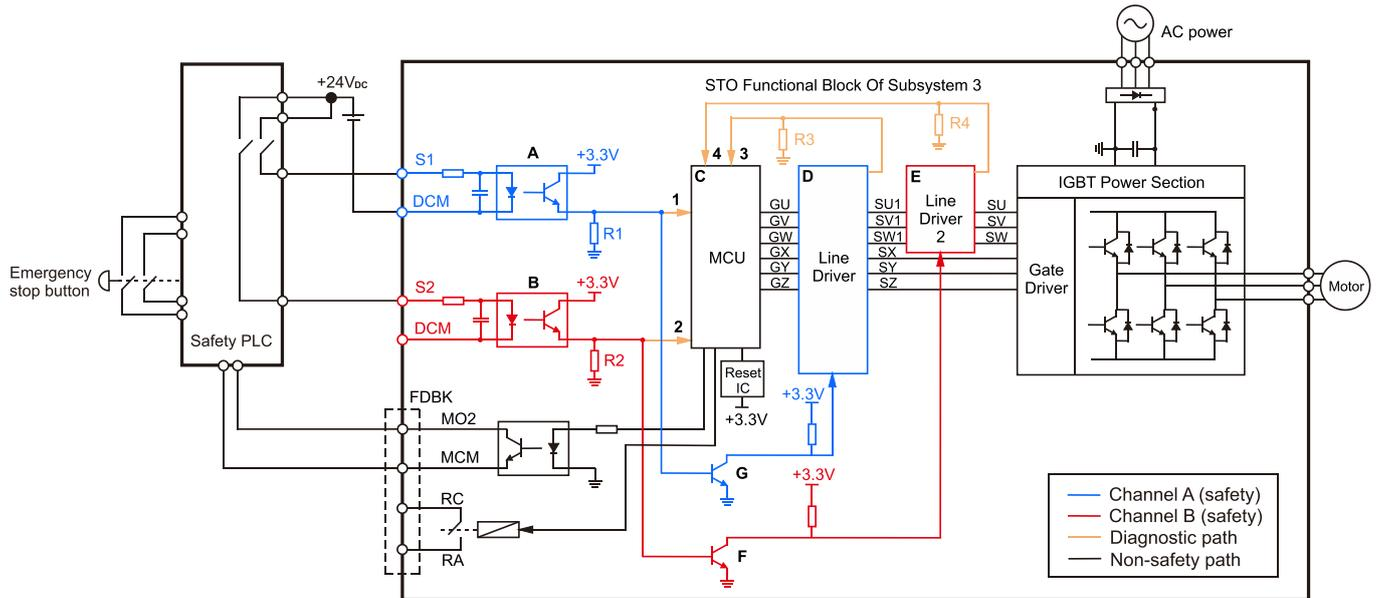
Figure 17-1: The circuit diagram for the Safe Torque Off function
