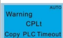
If you unplug the keypad and plug it back while copying the PLC program, the screen displays a CPLt warning.
