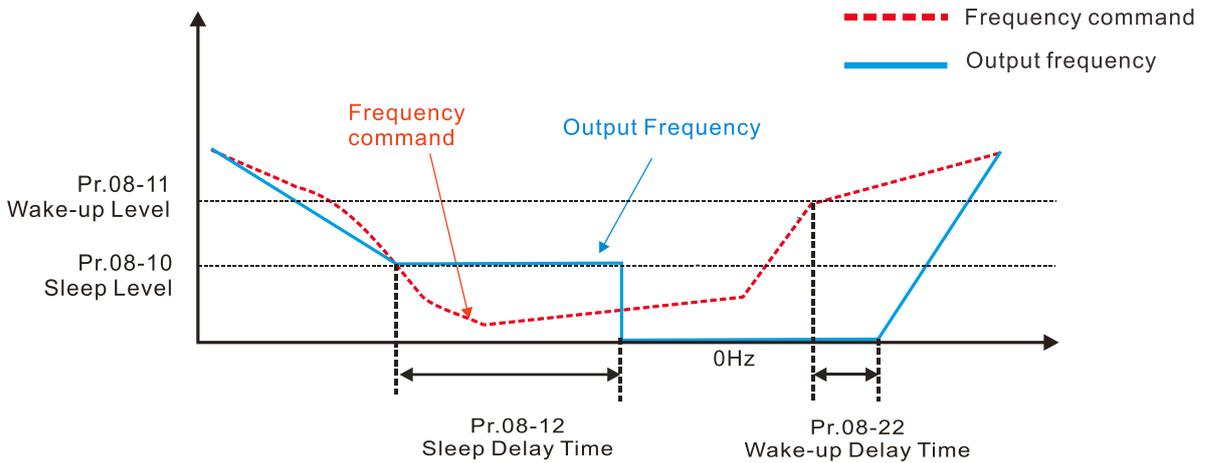
2. **Internal PID Calculation Frequency Command (PID is in use, Pr.08-00 ≠ 0 and Pr.08-18=0.)**
