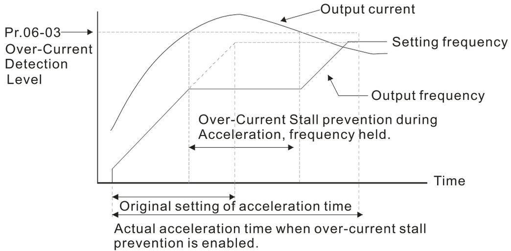
Refer to Pr.06-16 for the stall level in flux weakening region. The protection curve:
