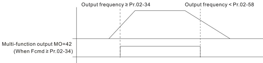
📖 It is recommended that you use this with the Dwell acceleration/deceleration function as shown in the following diagram.
