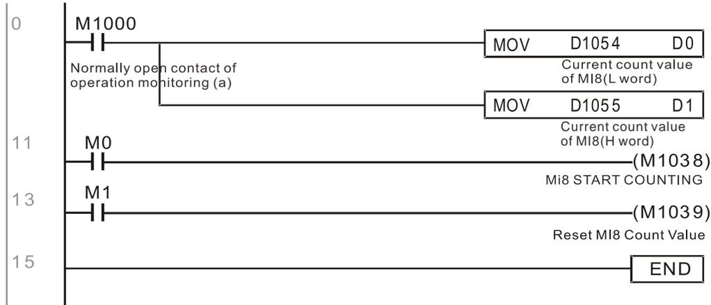
**NOTE:** When the PLC program defines MI7 for use as a high-speed counter, that is, when M1038 or M1039 is written in PLC procedures, other functions of MI7 are disabled.
