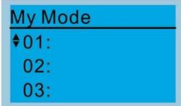
Press F4 in parameter setting screen to save the parameter to My Mode. To delete or
