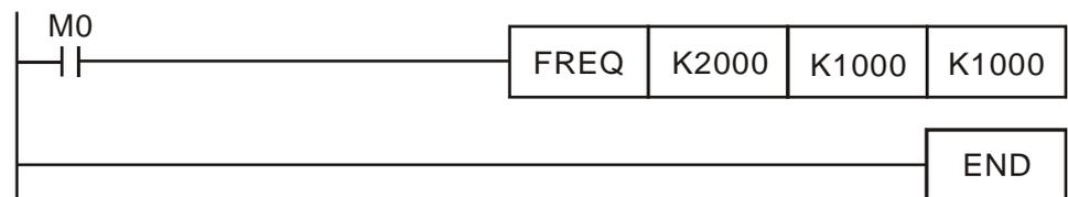
If we force M0 to 1, the frequency command is 20.00 Hz; but when M0 is set to 0, there is a different situation.
