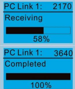
Start to upload parameters to VFDSOft.
