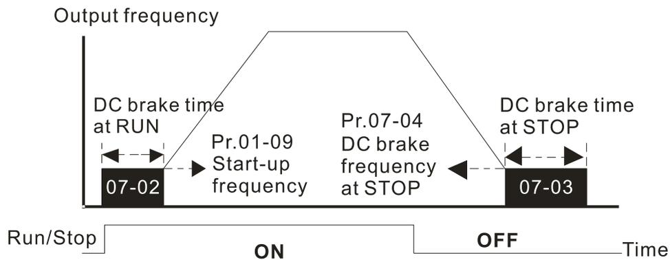
DC Brake Output Timing Diagram
