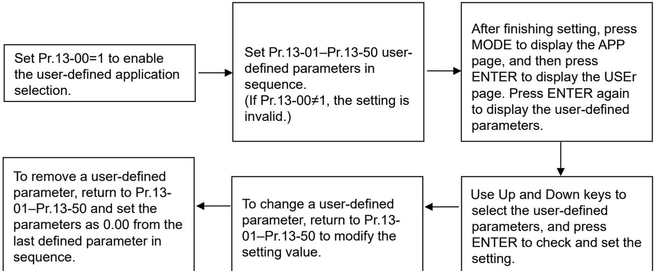
1. Use Pr.13-01–Pr.13-50 to set the user-defined parameters in sequence according to your requirement. The default setting 0.00 means there is no user-defined parameter. Press ENTER to set the corresponding parameters for Pr.13-01–Pr.13-50.
