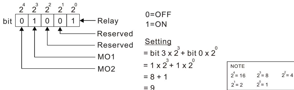
**02-52** Display the External Multi-function Input Terminals Used by PLC
