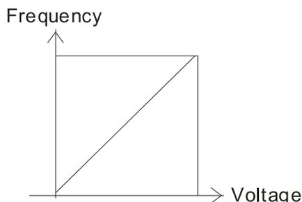
$$F_{cmd} = [(ay \pm bias) \times gain] \times \frac{F_{max}(01-00)}{10V \text{ or } 16mA \text{ or } 20mA}$$
