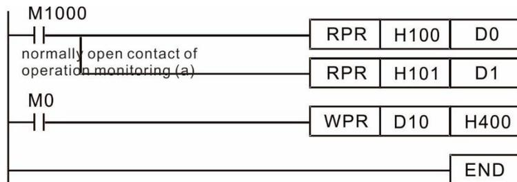
Recommendation: Be cautious when using the WPRA command. When writing parameters, most parameters are recorded when they are written, and these parameters may only be revised  $10^6$  times: a memory write error may occur if parameters are written more than (MS) $10^6$  or (MH) $10^9$  times.
