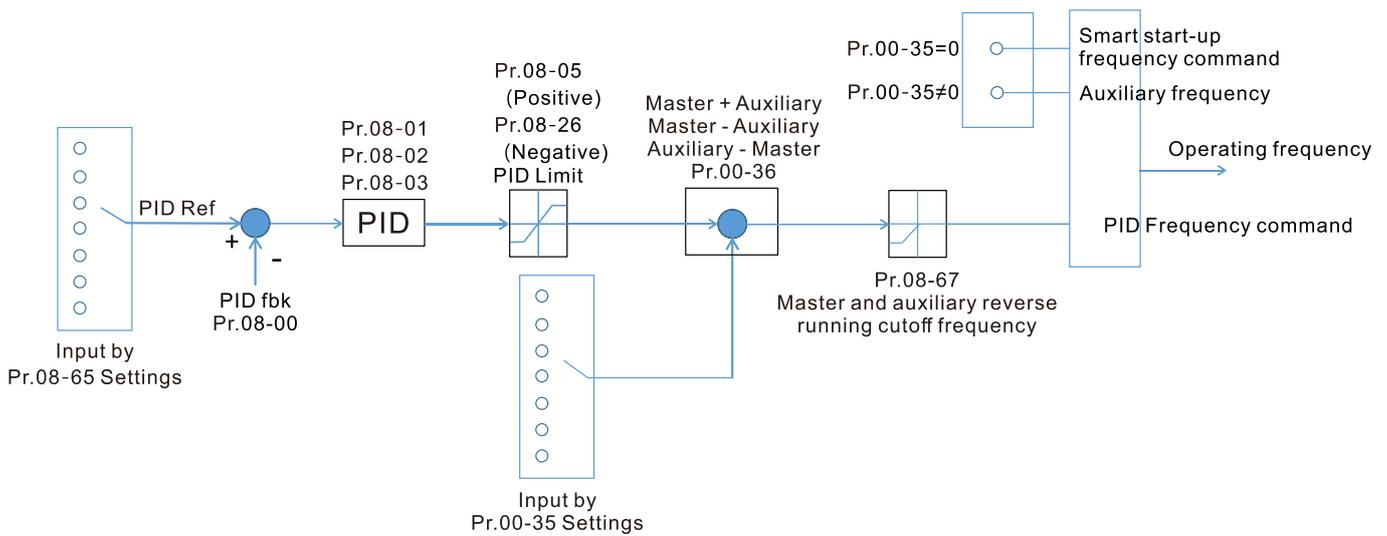
When Pr.08-65 ≠ 0, the PID controller architecture shows as the diagram below:
