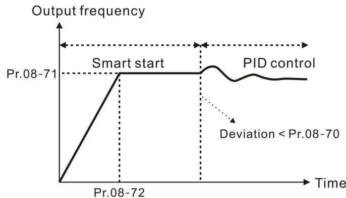
✎ **08-75** PID2 Parameter Switch Condition
