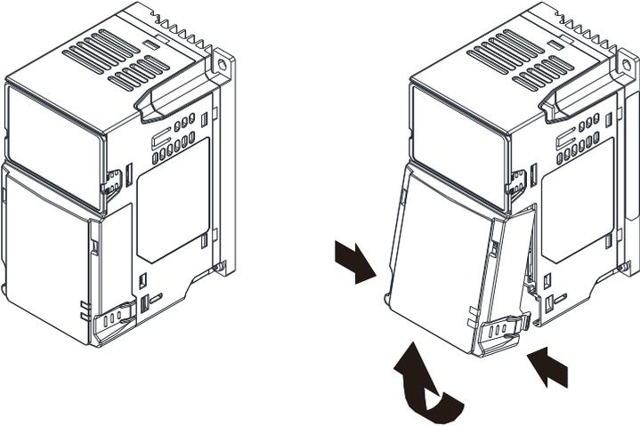
Press the clip on both sides, and then remove the cover by rotating it.
