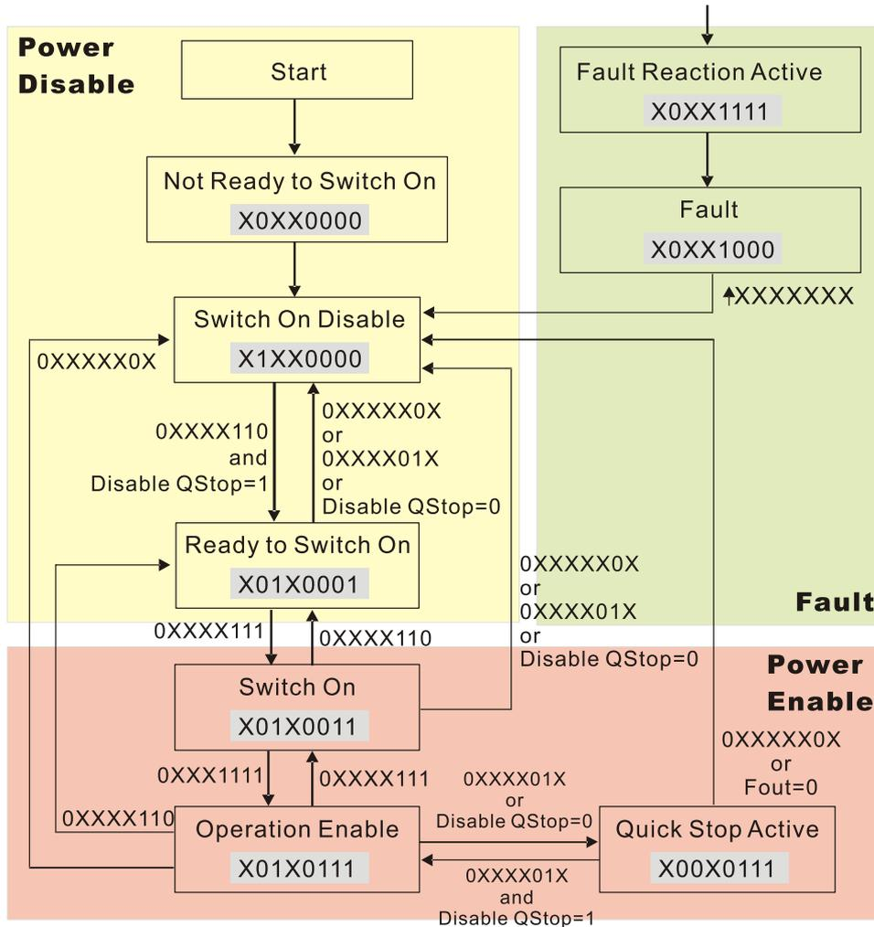
Set command 6040 = 0xE, and then set another command 6040 = 0xF. Then you can switch the motor drive to Operation Enable. The Index 605A determines the direction of the lines from Operation Enable when the control mode changes from Quick Stop Active. When the setting value is 5-7, both direction lines are active, but when the setting value of 605A is not 1-3, once the motor drive is switched to Quick Stop Active, it is not able to switch back to Operation Enable...
