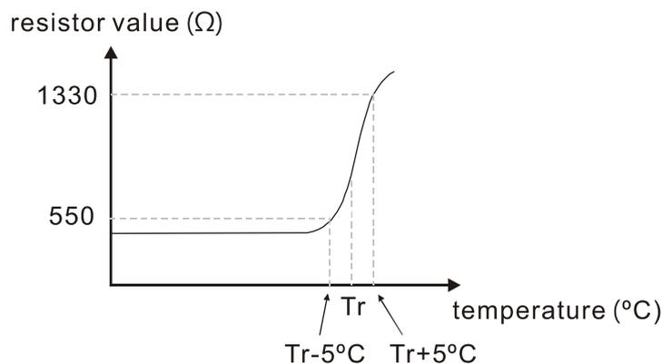
Refer to the following calculation when Pr.06-30 is set to 23% and motor temperature overheating protection level is 1330 Ω:
