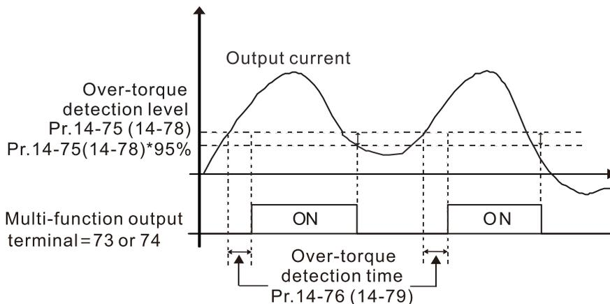
When you set Pr.14-74 or Pr.14-77 to 2 or 4, an ot3/ot4 warning displays and the drive stops running after over-torque detection. The drive does not run until you manually reset it.
