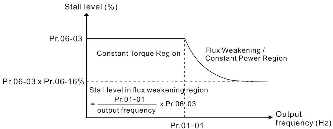
When you enable the over-current stall prevention, the drive's acceleration time is longer than the setting.
