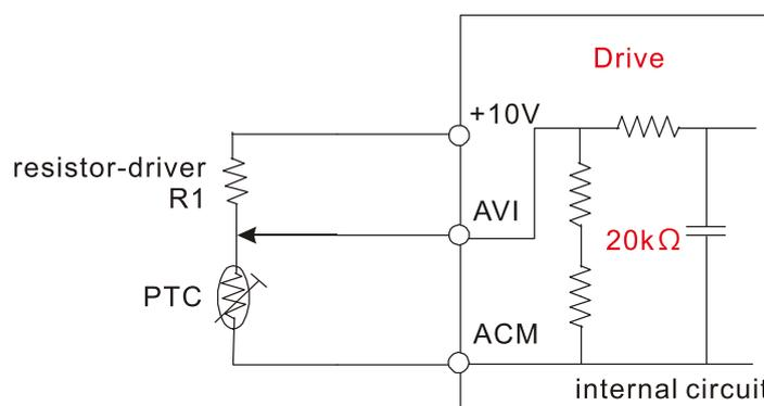
Take the standard PTC thermistor as an example: if the protection level is 1330 Ω, the actual voltage between +10V-ACM is 10.5 V and divider resistance R1 is 4.4k Ω.
