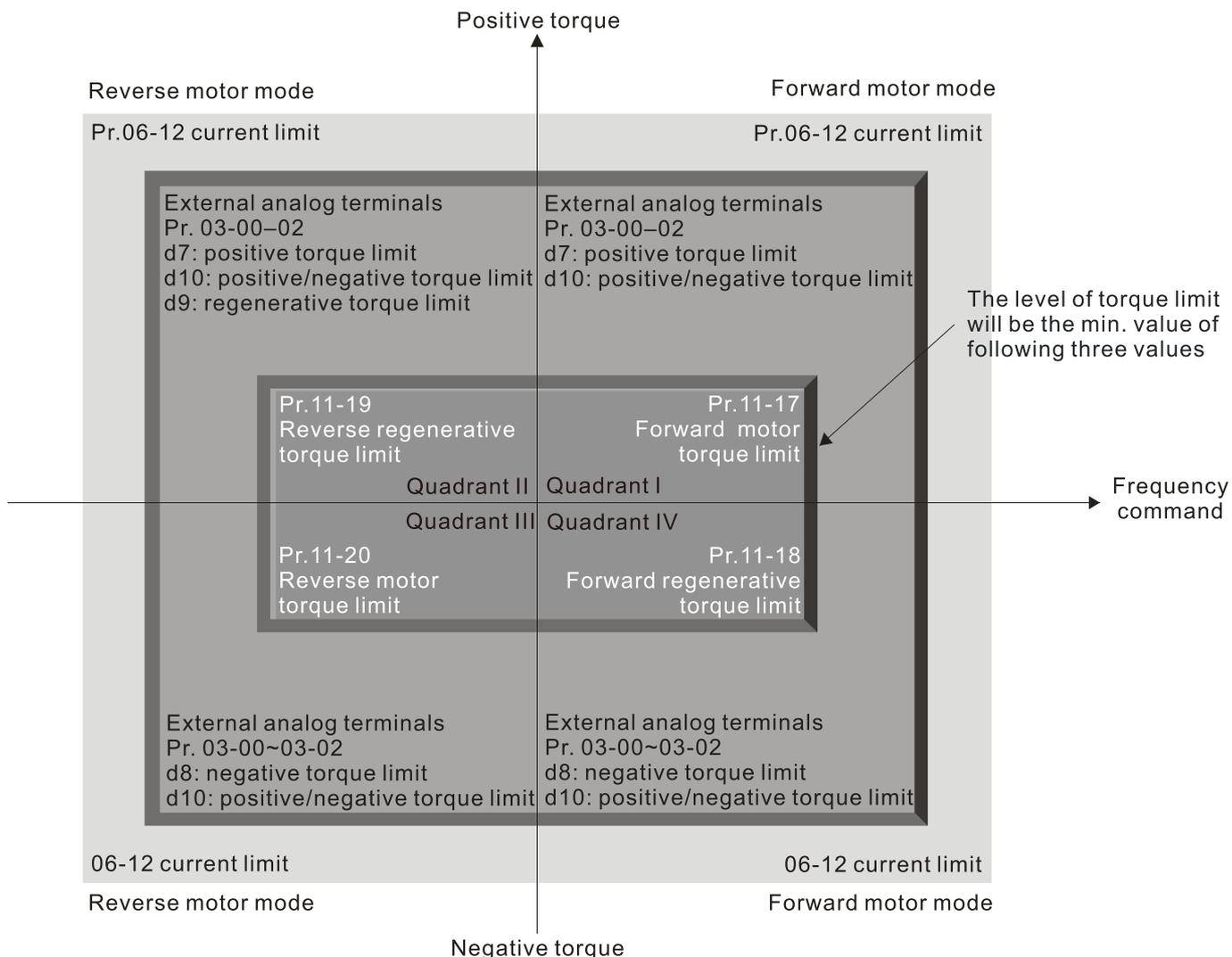
📖 All control modes are based on 100% of the motor rated current except:
