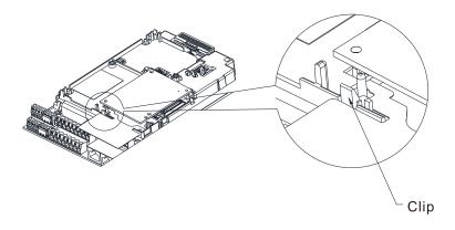
Twist to open the other clip to remove the PCB.
