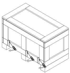
2. Remove the cover of wood box and then take out the EPE tray and user manual.
