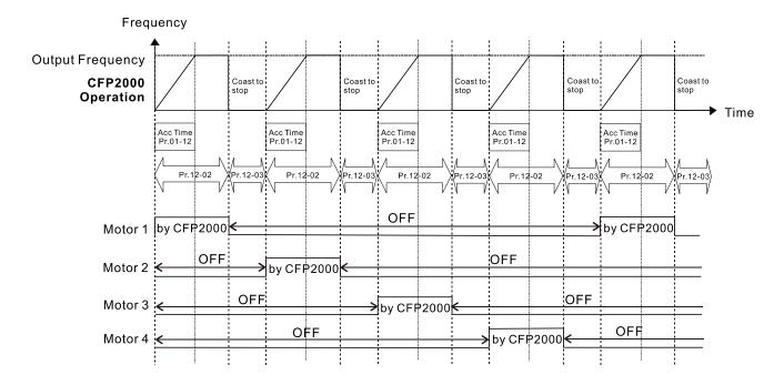
Diagram 12-1: Sequential Diagram of Fixed Time Circulation Free Running Mode (by time)
