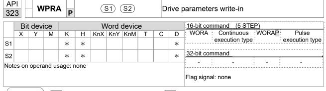
S1: Data that is going to write in S2: Parameter address of the write-in data
