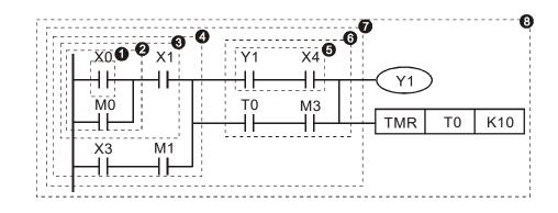
Explanation of basic structure of ladder diagrams
