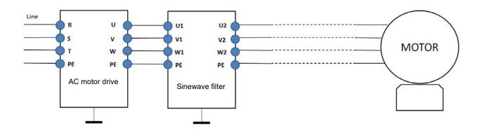
Wiring of non-shielded cable
