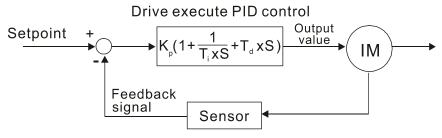
$K_p$ : Proportional gain (P)  $T_i$ : Integral time (I)  $T_d$ : Derivative control (D) S: Operator
