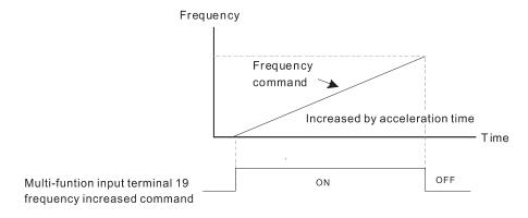
When Pr.02-09 is set to 1: the increasing / decreasing frequency command (F) operates according to the setting for Pr.02-10 (0.01–1.00 Hz/ms).
