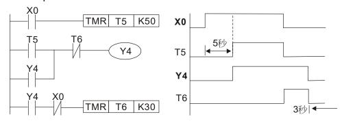
Example 12: Extended timing circuit
