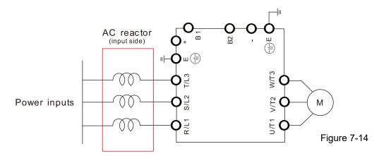
Wiring an AC input reactor
