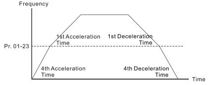
1st/4th Acceleration/Deceleration Frequency Switching
