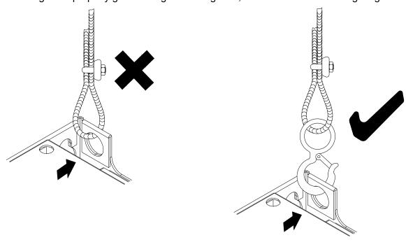
Ensure the angle between the lifting holes and the lifting device is within the specification, as shown in the following figure.
