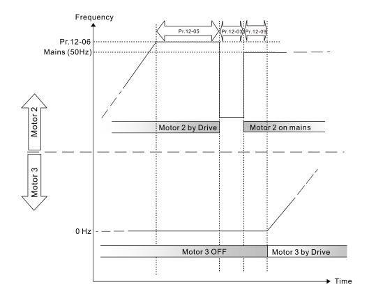
Diagram 12-15 Sequence of Fixed Quantity Circulation Output Delay
