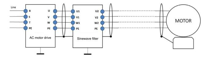
Wiring of shielded cable
