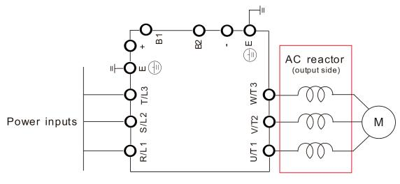
Wiring an AC output reactor
