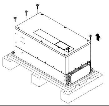
4. Lift up the drive by using hooks through the holes.
