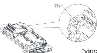
Twist to open the other clip to remove the PCB, as shown in the figure on the left.
