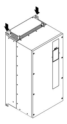
Ensure the lifting hook properly goes through the lifting hole, as shown in the following diagram.
