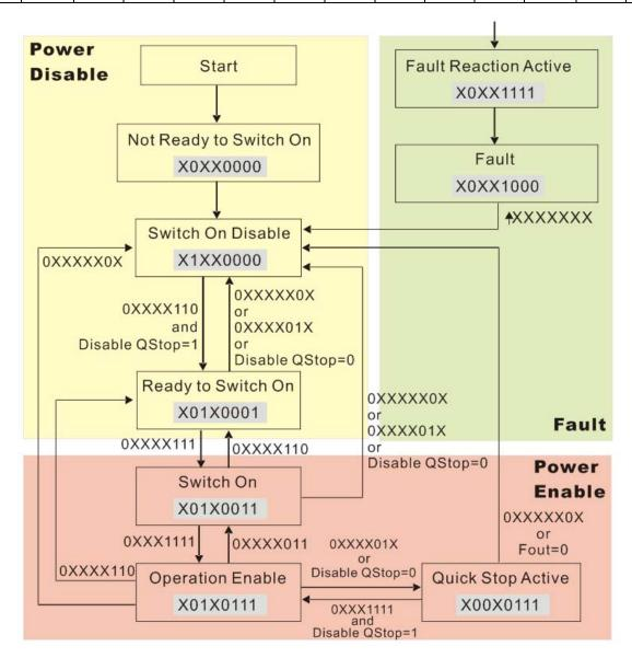
Set command 6040=0xE, then set another command 6040 =0xF. Then you can switch the motor drive to Operation Enable. The Index 605A determines the lines from Operation Enable when the control mode changes from Quick Stop Active. When the setting value is 1–3, both lines are active, but when the setting value of 605A is not 1–3, once the motor drive is switched to Quick Stop Active, it is not be able to switch back to Operation Enable.
