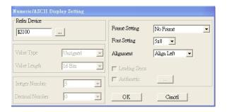
Related Device: Choose the VFD Communication Port that you need, if you want to read output frequency (H), set the VFD Communication Port to \$2202. For other values, please refer to ACMD Modbus Comm Address List.
