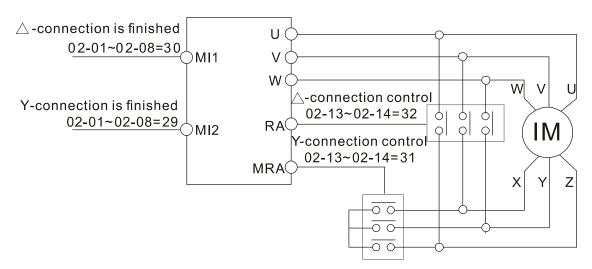
Y-△ connection switch: can be used for wide range motor
