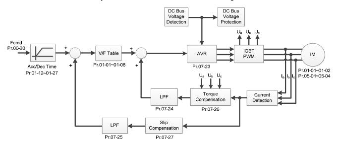
When Pr.00-10=0, and you set Pr.00-11 to 2, the space vector control diagram is as follows. Induction Motor Space Vector Control (IMSVC)
