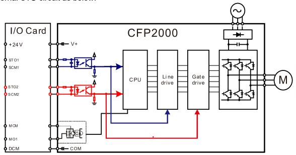
18-3-2 In the figure below, the default setting for +24V-STO1-STO2 and SCM1-SCM2-DCM is short circuit:
