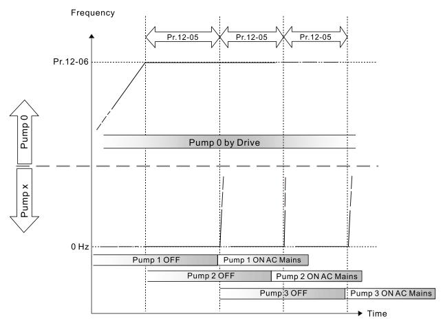
Diagram 12-9: Sequence of switching motors at Fixed Quantity Control with PID
