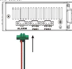
A typical way to use the alarm is to connect the Alarm circuit to a warning light or buzzer in the control room. The light or buzzer could be set up to turn on when any of the above two conditions is detected.
