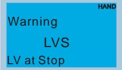
The image shows a blue rectangular display area with white text. The text is arranged vertically: "Warning" at the top, "LVS" in the middle, and "LV at Stop" at the bottom. In the top right corner of the blue area, the word "HAND" is written in a smaller font. | While stopped, the power feedback unit detected voltages lower than the value set in parameter 03-00 on the high-voltage end of the internal DC voltage. |
