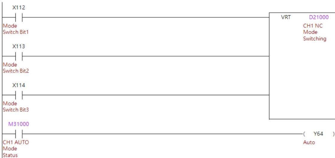
Figure 6.1.3 Mode switching by knob
