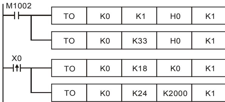
1. Write H'0 into CR#1 of analog input module No. 0 to set CH1 as mode 0 (voltage input: -10V ~ +10V).
