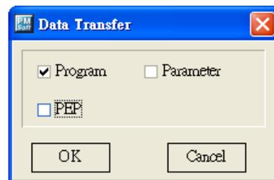
2. Check “PEP” to read the protection area and click “OK”, as a.). Next, enter the password and confirm it, as b.), to start uploading general program, protected program and E-CAM data to PC, as c.).
