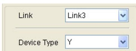
Design the buttons Y0~Y7 for both DVP-PM according to the above procedure as the diagram below. Buttons Y0~Y7 correspond to Y0~Y7 of Link3 (Slave1) and Link4 (Slave2). When the above settings are completed, the Ethernet connection between HMI and the 2 DVP-PM can be performed.
