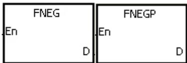
**D** : Device in which the sign of the value is reversed
