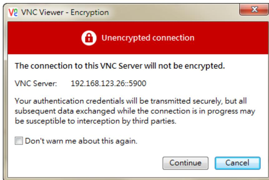
But if connection is failed, it will appear the following window. It means the IP address does not exist or the VNC network application is not enabling.
