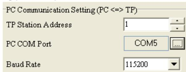
6. TP70P can communicate with the computer by means of the communication port. TPEditor is used to upload/download a text panel program, and WPLSoft is used to upload/download/monitor a PLC program.
