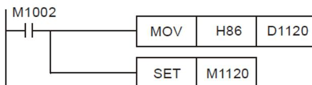
**Example: COM2 uses RTU communication.**
