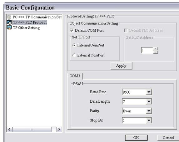
**Step 4:** Compile the program created, and download the program to TP70P. Connect COM3 on TP70P to an RS-485 communication port on a PLC.
