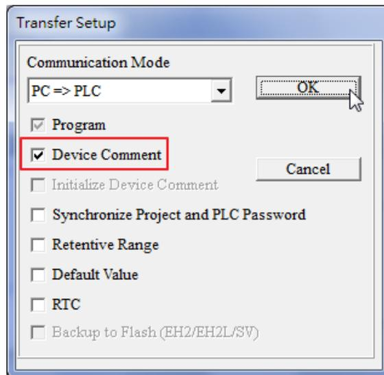
After the users select the **Device Comment** checkbox, the **System Block** window will appear. The users can select devices and set device ranges.
