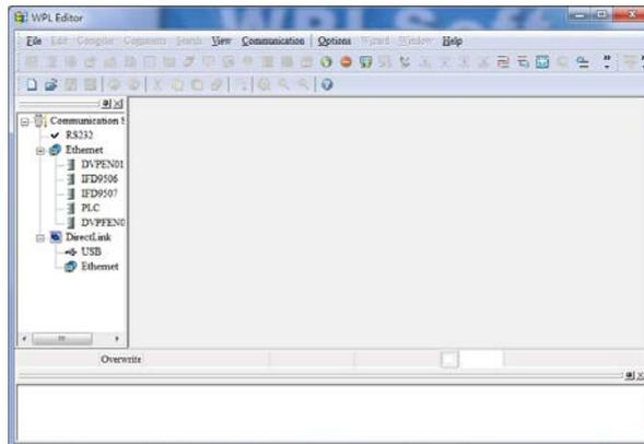
Step 2: After
