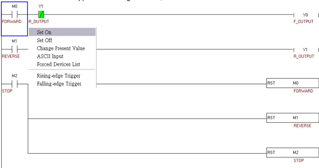
Note: **Set On** and **Set Off** can not be used to change the state of a device corresponding to an actual I/O device because the state of the actual I/O device immediately overwrites the value which is set. **Force ON** and **Force OFF** can be used instead.
