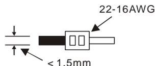
The torque applied to the screws on TP70P should be 1.90 kg-cm (1.65 in-lbs). Only copper leads which can resist the heat above 60°C/75°C can be used.
