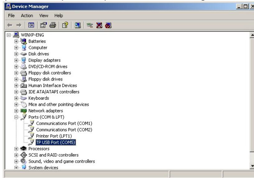
5. The communication port which is connected to TP70P is also shown in the **PC COM Port** box in the **PC Communication Setting (PC <=> TP)** section in TPEditor.
