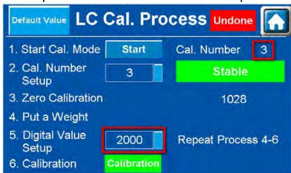
**(7)** After all calibrations are complete, the LC Cal. Process condition shown in the upper right corner changes from **Undone** in a red block to **Done** in a green block. Press **Storing Data** in the lower right corner to save the settings. Otherwise, the changes will not be saved. Press **Default Value** in the upper left corner to cancel without saving the changes. You can always reset calibrations to default settings by pressing **Default Value** in the upper left corner.
