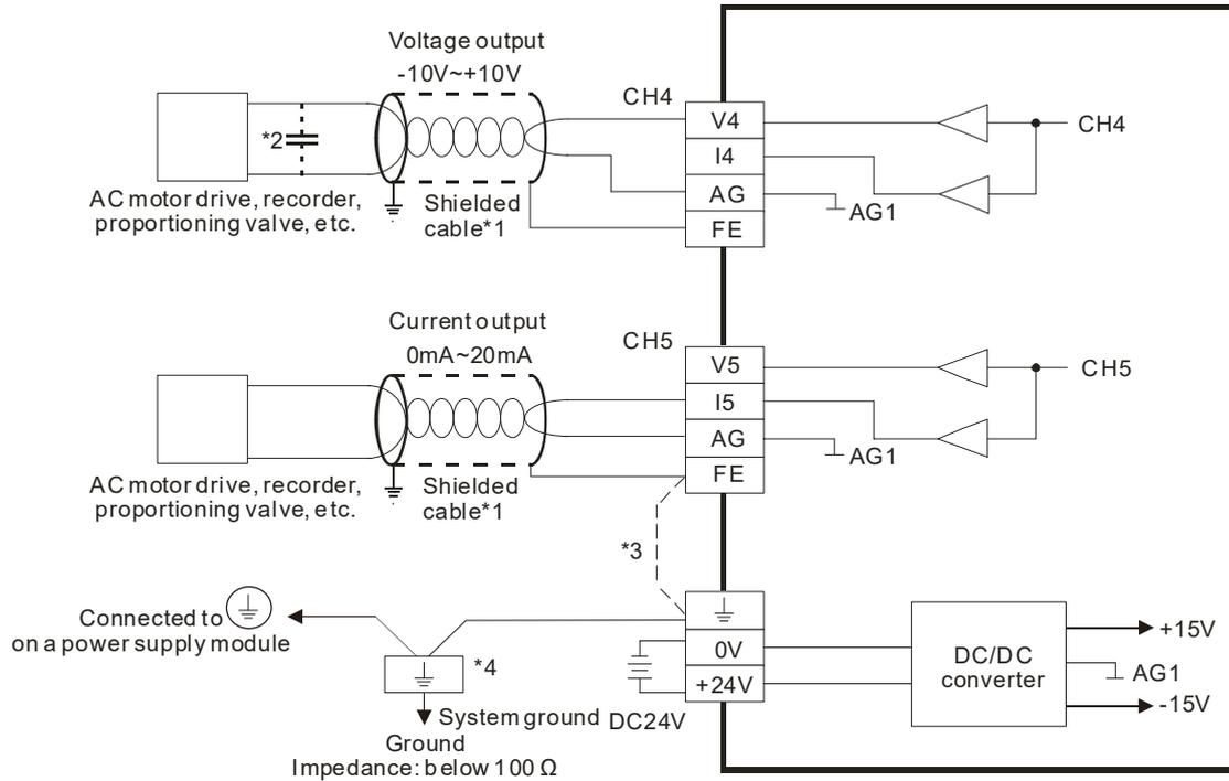
\*1. Use shielded cables to isolate the analog input signal cable from other power cables.
