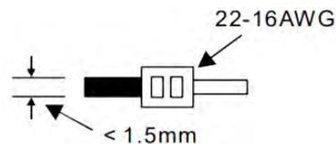
2. For power terminals, use single-core cables or twin-core cables in a diameter of 12 AWG–22 AWG. Use only copper conducting wires that can resist temperatures above 60° C–75° C. The required torque for tightening a PLC terminal screw should be less than 5–8 kg-cm (4.3–6.9 lb-in).
