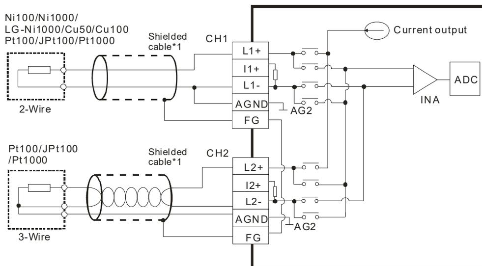
\*1. Use shielded cables to isolate the analog input signal cable from other power cables.
