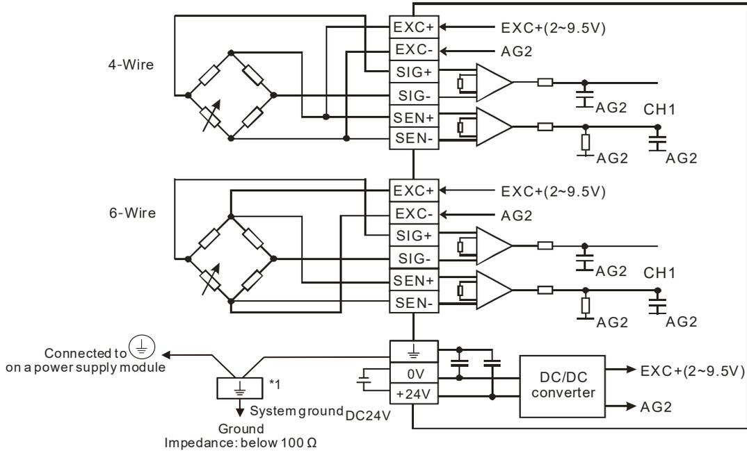
\*1. Connect the  $\perp$  of a power supply module and the  $\perp$  of the load cell terminal FE to the system ground and then ground the system ground or connect the system ground to a distribution box
