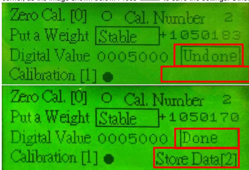
Use  to go back to the main setting menu and you can see the status shown is **Finish** as the image shown below. This indicates the calibration is complete.
