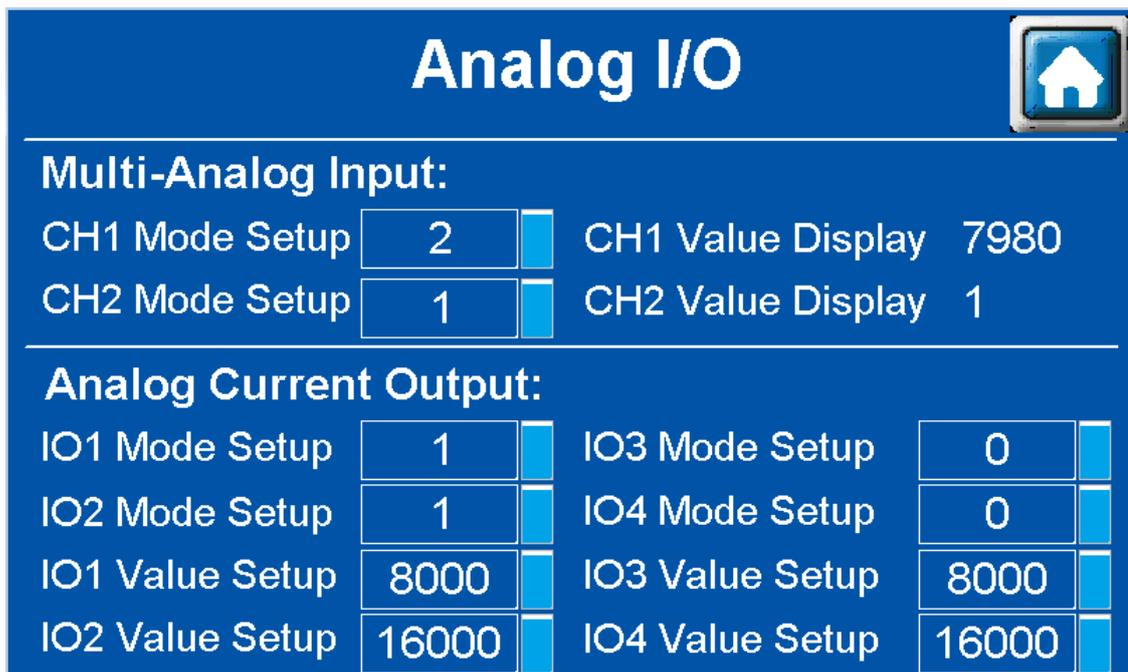
TP70P-211LC1T is with two-channels of multi-analog inputs and four-channels of analog current outputs. You can set up different modes for each channel, read input values and set up output values under this setting item. You can perform basic operations including system adjustments and checks before you have your own programs ready.
