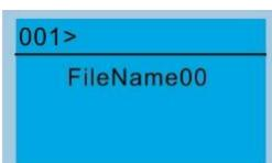
Press the Up / Down keys to select a symbol. Press the Left / Right keys to move the cursor to select a file name.
