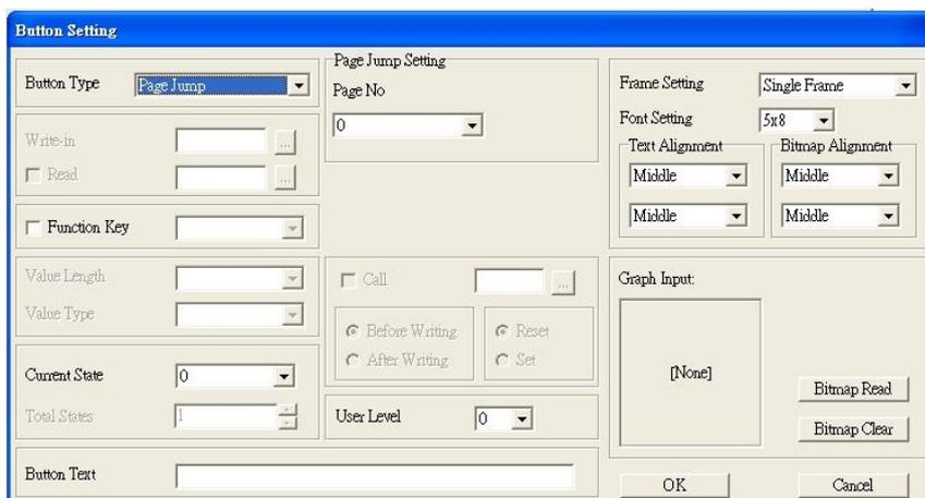
**Button Type:** specifies the button’s functions. Page Jump and Constant Setting are the only functions currently supported.
