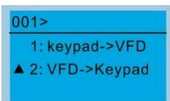
Press ENTER to go to the “VFD→Keypad” screen.
