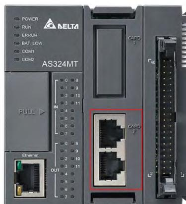
Note: the AS-FCOPM card can only be installed in the Card 2 slot in the AS series
