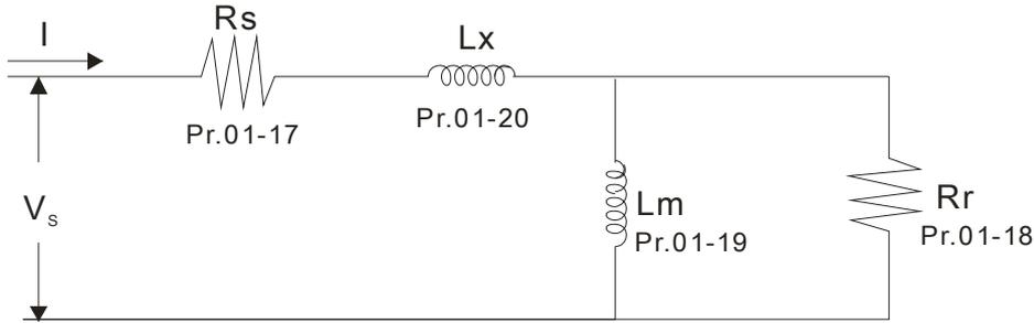
※ When Pr.01-11 is set to 2 (static test), user needs to write no-load current value of motor into Pr.01-16.
