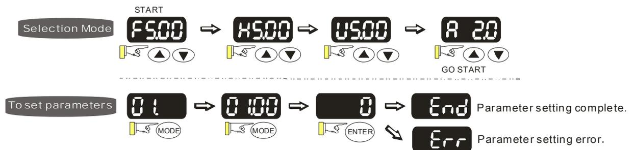
NOTE: In the parameter setting mode, user can return to MODE selection by pressing (MODE).
