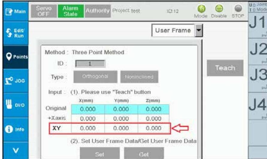
**Figure 2-20 Point information - Setting up XY or +Y point for the user coordinates (+Yaxis direction)**
