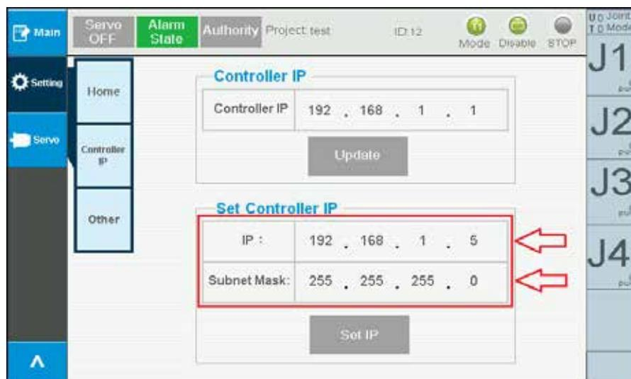
Figure 2-37 System setting - Setting controller IP
