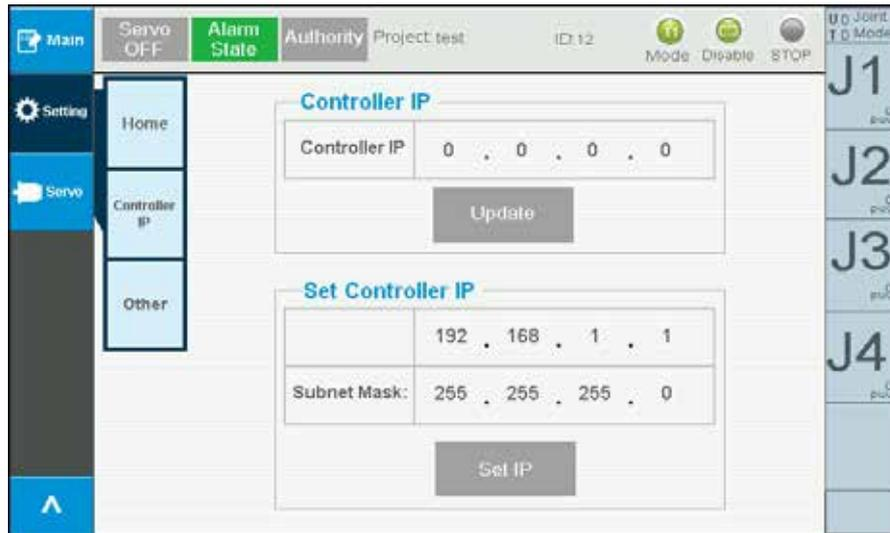
Figure 2-35 System setting - Controller IP
