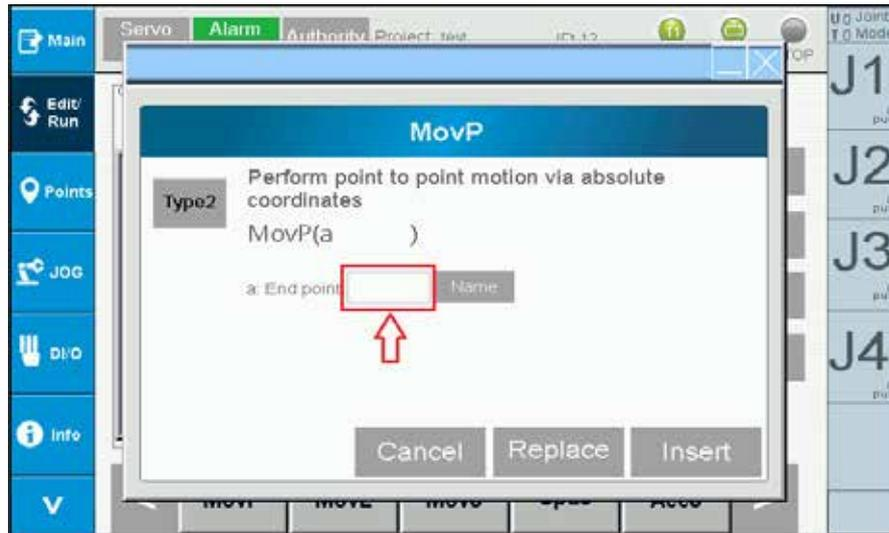
Figure 2-12 Edit/run program for robot - Enter command name and other information
