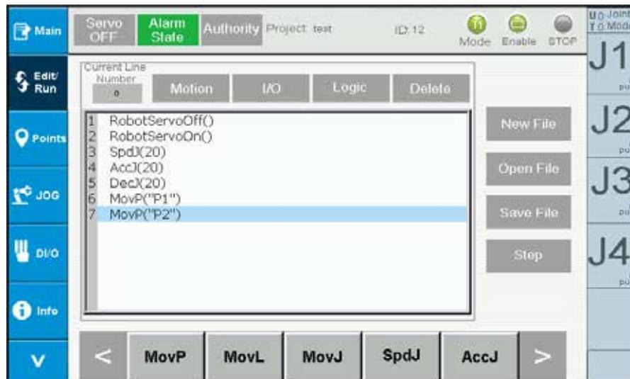
Figure 2-8 Edit/run program for the robot - Project opening completed
