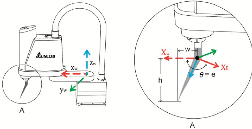
Figure 2-21 Tool size Height, Width and Degree
