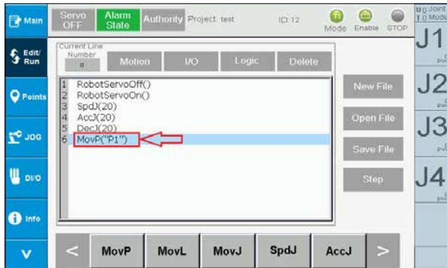
Figure 2-9 Edit/run program for the robot - Select input position
