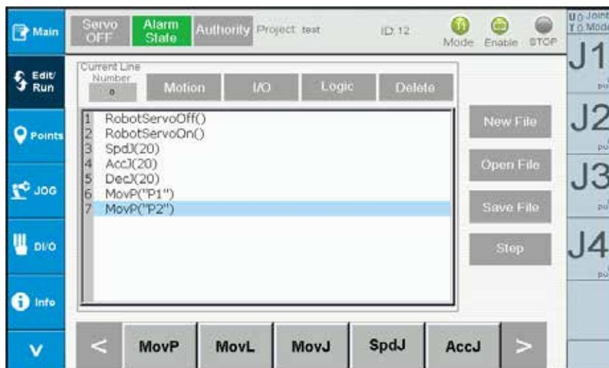
Figure 2-13 Edit/run program for robot - Input completed
