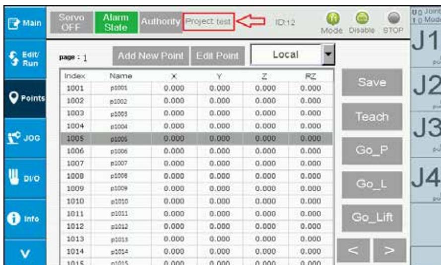
Figure 2-16 Point information - Local point operation for the test project
