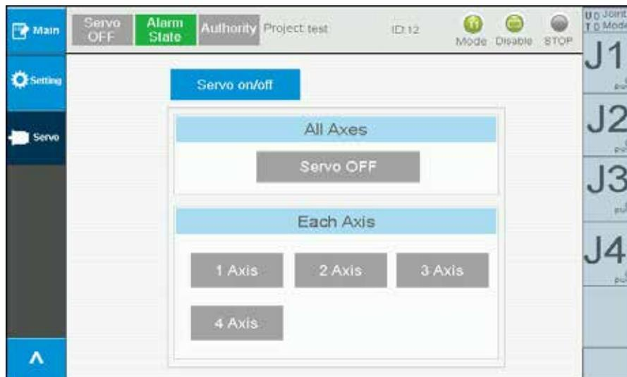
Figure 2-38 Servo Setting Servo On/Off
