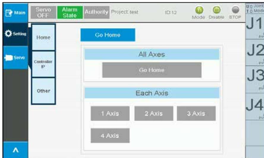
Figure 2-34 System setting - Returning to original point
