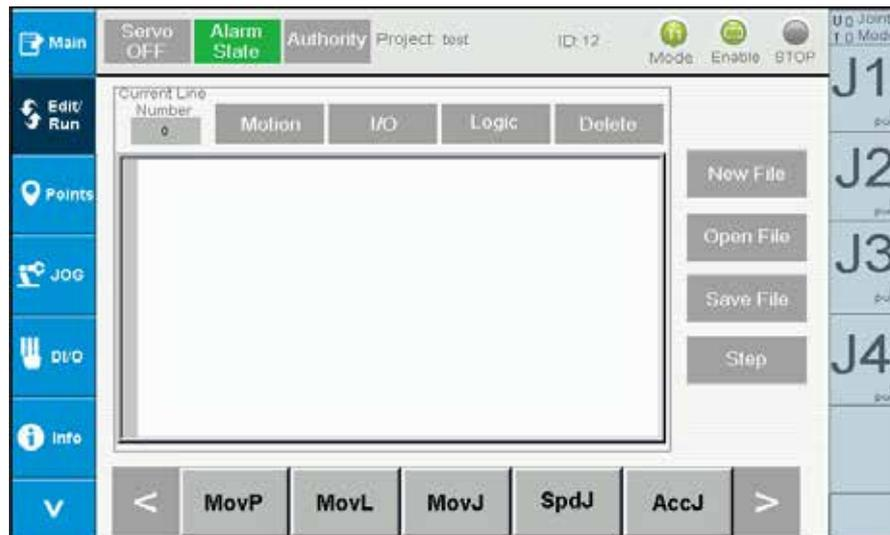
Figure 2-6 Edit/run program for the robot - Creation of new project completed
