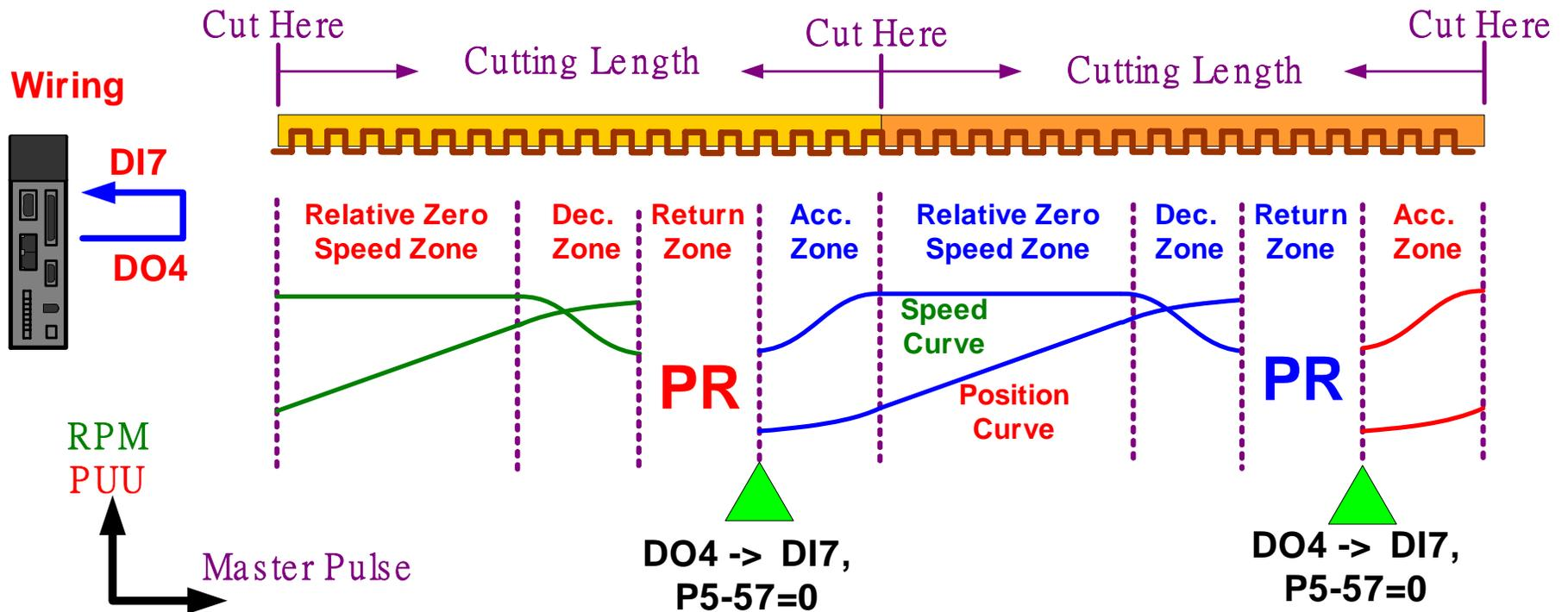
Compare data array: The pulse number of cutting length.
