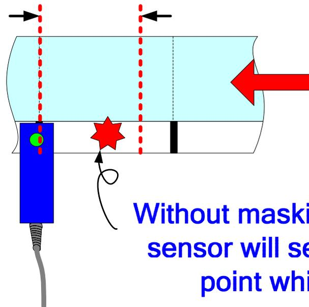
Without masking function, the mark sensor will send signal out at this point which is unwanted.
