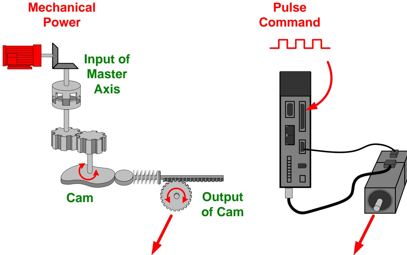
If both of the axes work in the same manner, the Servo system can be used to replace the mechanical CAM.
