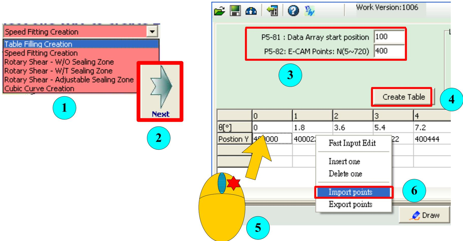
The screenshot illustrates the 'Table Filling Creation' process in a software application. The interface is annotated with numbered callouts (1-6) and red boxes highlighting key elements.
