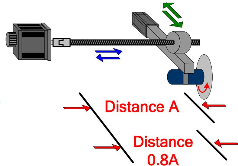
The relative zero speed zone will be shortened. Check if it is long enough for flying saw to finish cutting job.
